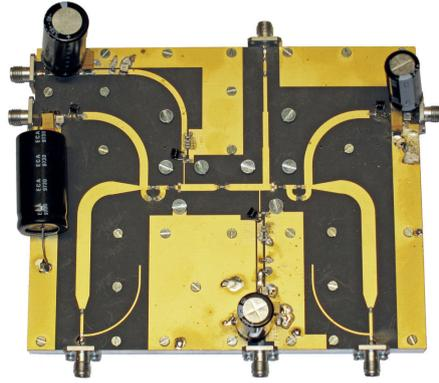
Figure 4.14: Photo of the dual RF-input 1.5–2.4 GHz hybrid circuit presented in [a,B].
