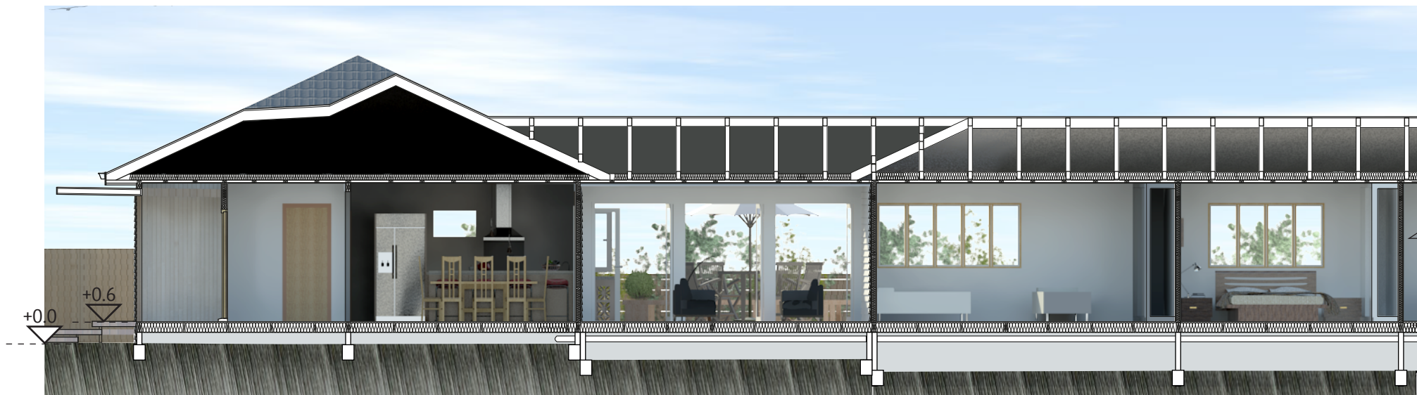
LONGITUDINAL SECTION (BB) THROUGH ENTIRE BUILDING PATIO 1600 ENTRANCE 2200 DINING 4200 INFORMAL LIVING 5500 BEDROOM 5600 BEDROOM 4000 27500 1m 5m
