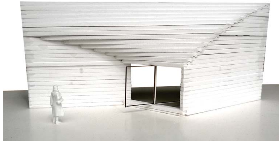
The original coggod dovetail is my point of departure and are adopted to the curved wall as well. The holes are for the tension rods.
