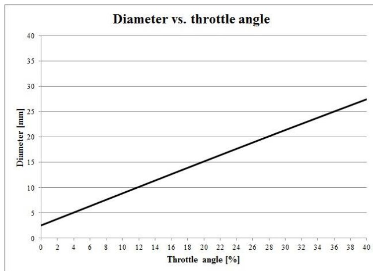
Figure 3.14. Relation between throttle angle and diameter.
