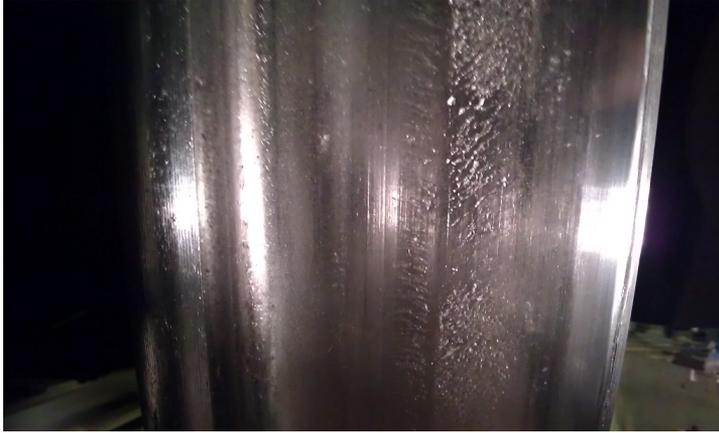
Figure 1.1: *Surface initiated rolling contact fatigue cracks on a loco wheel tread.*
