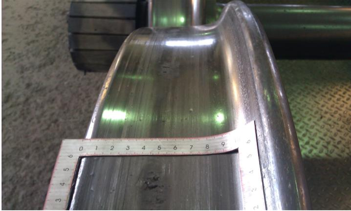
Figure 1.2: *Wagon wheel tread subjected to thermal and rolling contact loading, resulting in clustered thermomechanical damage.*
