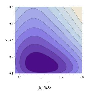
Figure 3.1: Illustration of the regularization using stochastic differential equation in the Lotka-Volterra predator-prey model. The two plots show the level curves of the objective function in the parameter estimation problem using the ordinary differential equation setting (a) and the stochastic differential equation setting (b). Note that in (a) there are several local minima to where an local optimization algorithm might converge.
