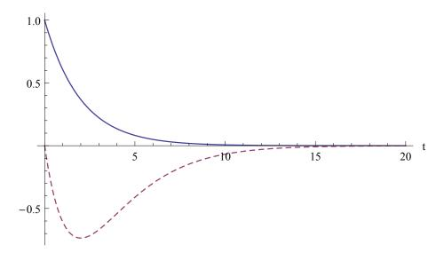
Figure 3.2: Illustration of sensitivity equations. The solution to the differential equation  $\frac{dA}{dt} = -kA$  (blue, solid) and its corresponding sensitivity with respect to the parameter k (purple, dashed). The initial condition is A(0) = 1 and the parameter value is k = 0.5.
