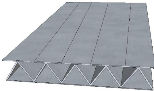
Figure 2.5 Geometry of a triangular truss core sandwich panel
