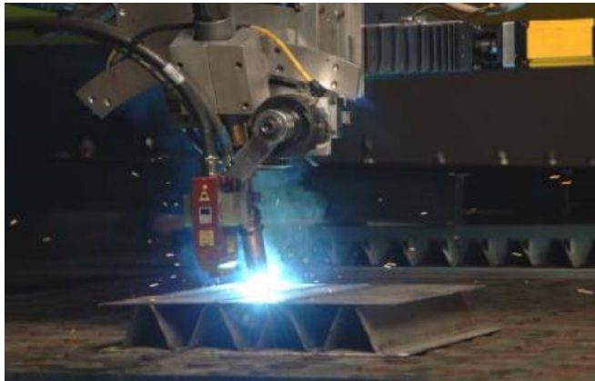
Figure 3.7 HLAW on a steel sandwich panel (SSP) (Defalco, 2007)
