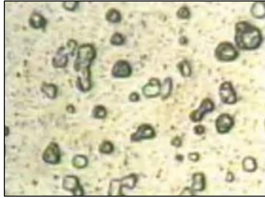
Figure 2.8: Example of pitting corrosion on a stainless steel sample. Note that the pitting corrosion is a localized corrosion phenomenon, whereas the intermittent surfaces remain largely intact. The sample metal is of the type Zeron 100. The sample is synthetically corroded in a lab environment (Comer, 2003).
