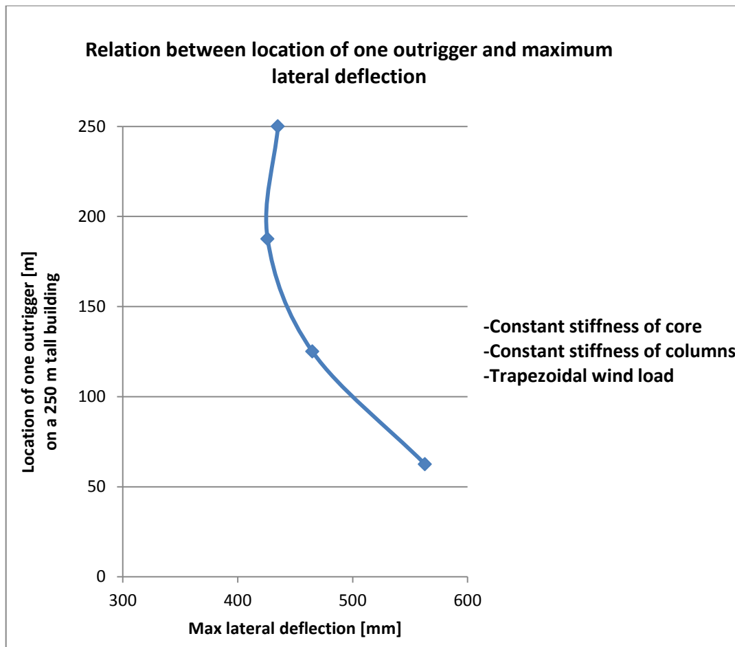
Figure 10.19: Relation between location of one outrigger and the maximum lateral deflection of a 245 m tall building with constant stiffness of the core.
