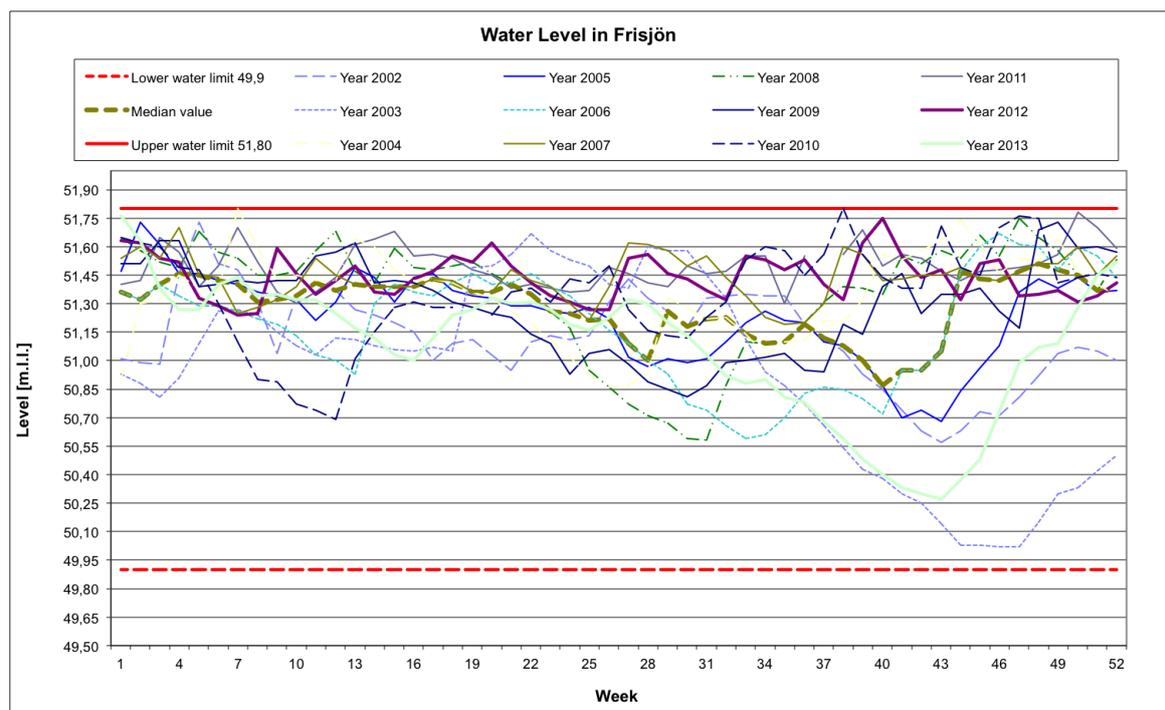
Figure 4.8: The water levels per week in Frisjön between 2004-2013. Height indicators refer to a local measure in meter based on a point in the area (Borås Energi och Miljö, 2013b).
