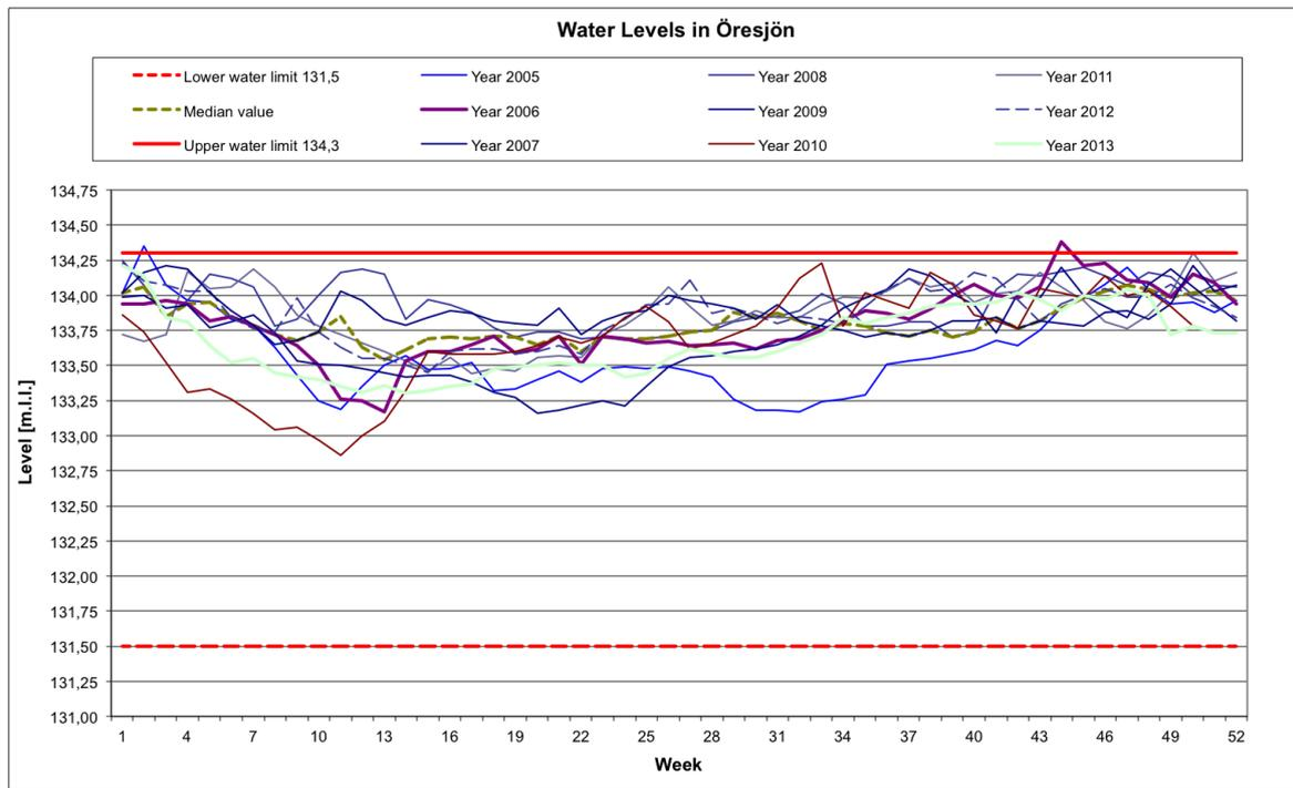
Figure 4.4: The water levels per week in Öresjön between 2008-2013. Height indicators refer to a local measure in meter based on a point in the area (Borås Energi och Miljö, 2013b).
