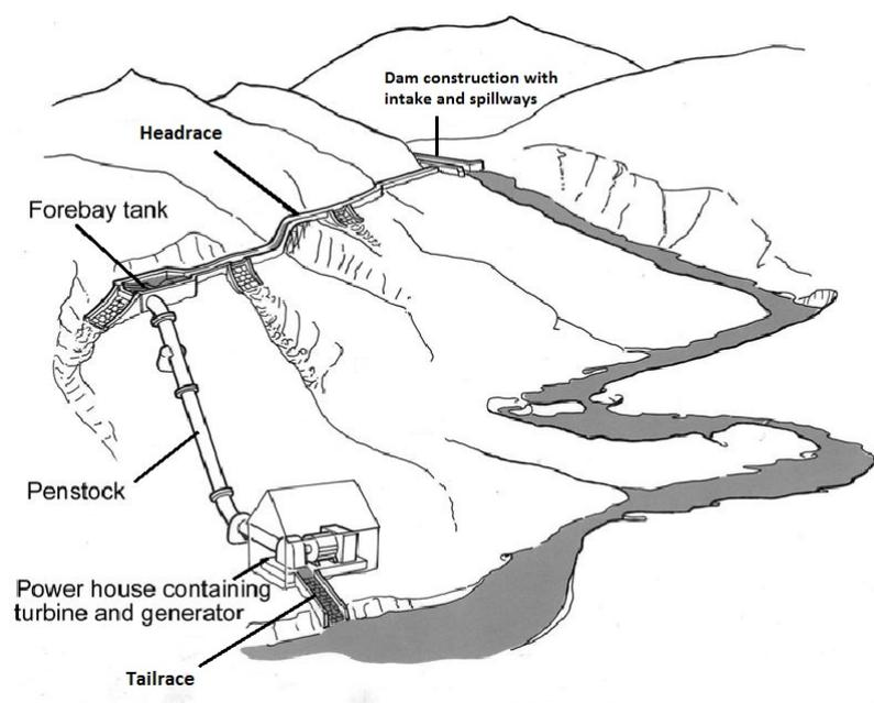
Figure 1.1: General components of a hydro power plant. The figure is based on the original picture from (Gatte and Kadhim, 2012)
