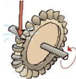
Figure 1.4: Pelton turbine (Sempler, 2009).
