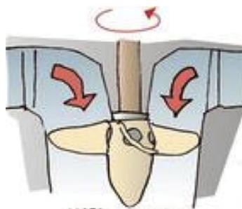
Figure 1.3: Kaplan turbine (Sempler, 2009).
