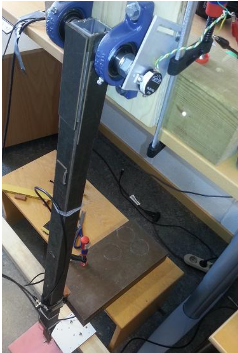
Figure 10. The constructed drop-test equipment.
