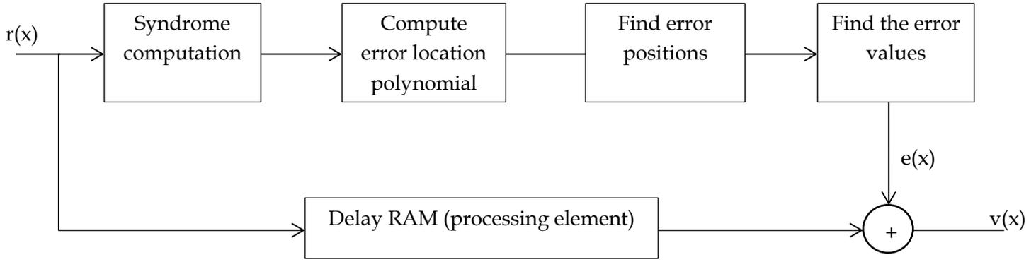
Figure 11. RS decoder with  $GF(2^m)$  arithmetic operations [5].
