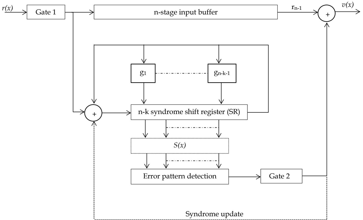
Figure 8. Meggitt Decoder for cyclic code [2].
