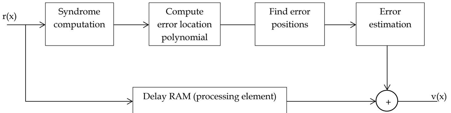
Figure 9. BCH decoder with  $GF(2^m)$  arithmetic operations [5].
