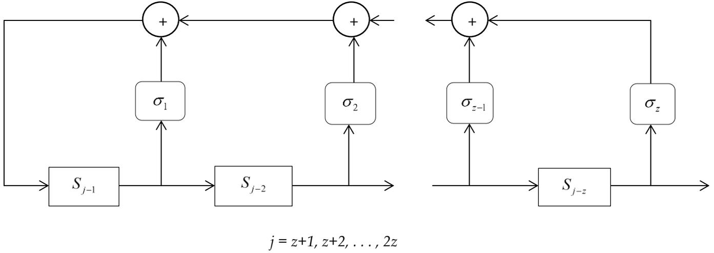
Figure 10. Linear Feedback Shift Register (LFSR)
