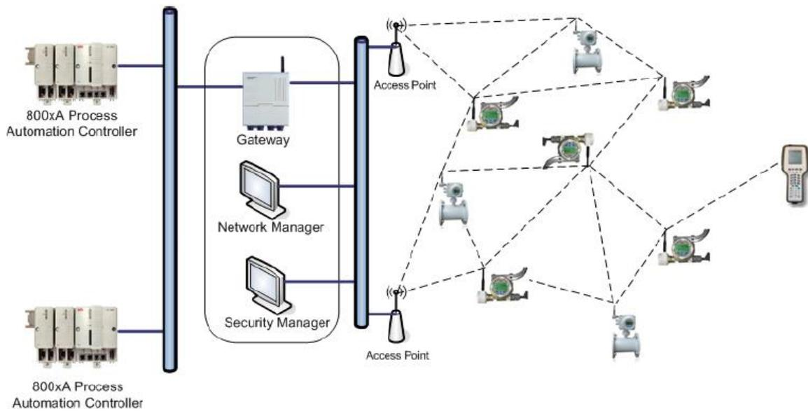
Figure 1. An industrial wireless sensor network structure
