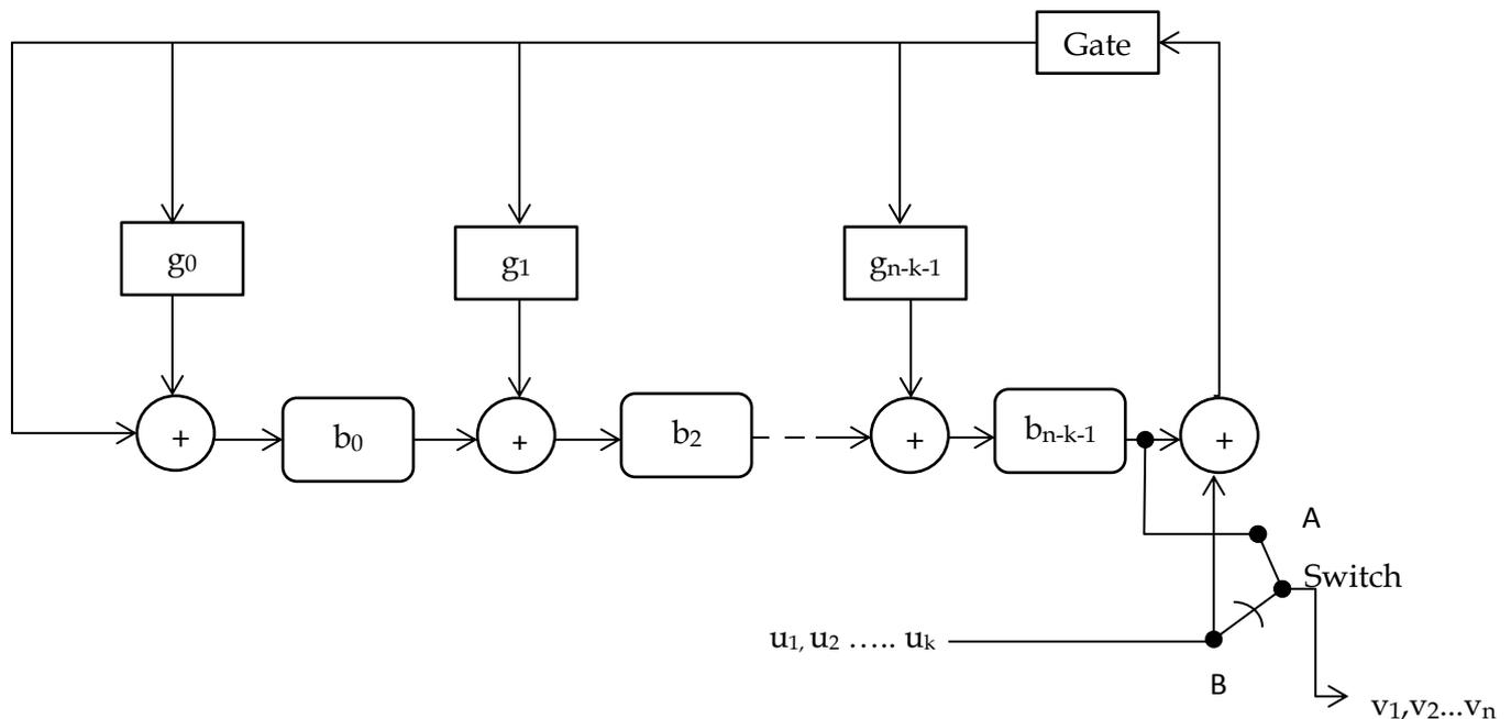
Figure 7. Shift Register Encoder.
