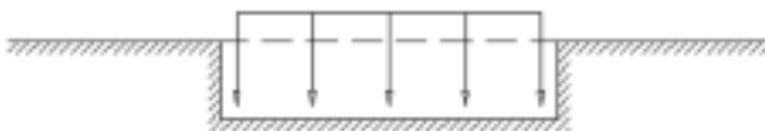
Figure 4.4 Load applied on a Winkler foundation (Based on Cook, 1999)
