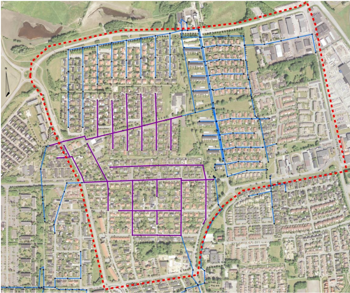
Figure 7.6 Purple lines are pipes to be relined in alternative 1
