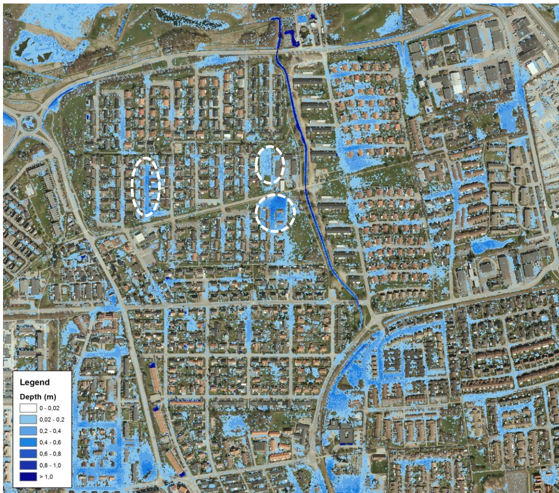
Figure 7.4 Water depth in closed areas
