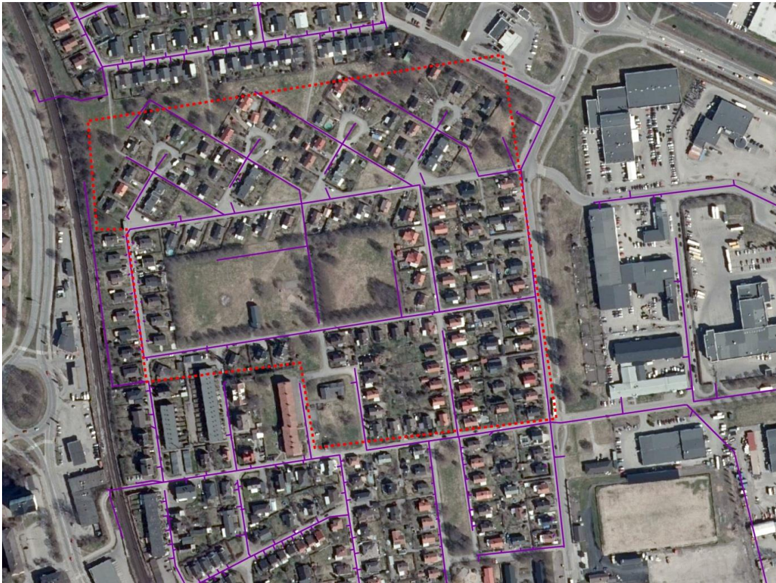
Figure 7.16 Sewer network (purple) within study area (red dashed line)
