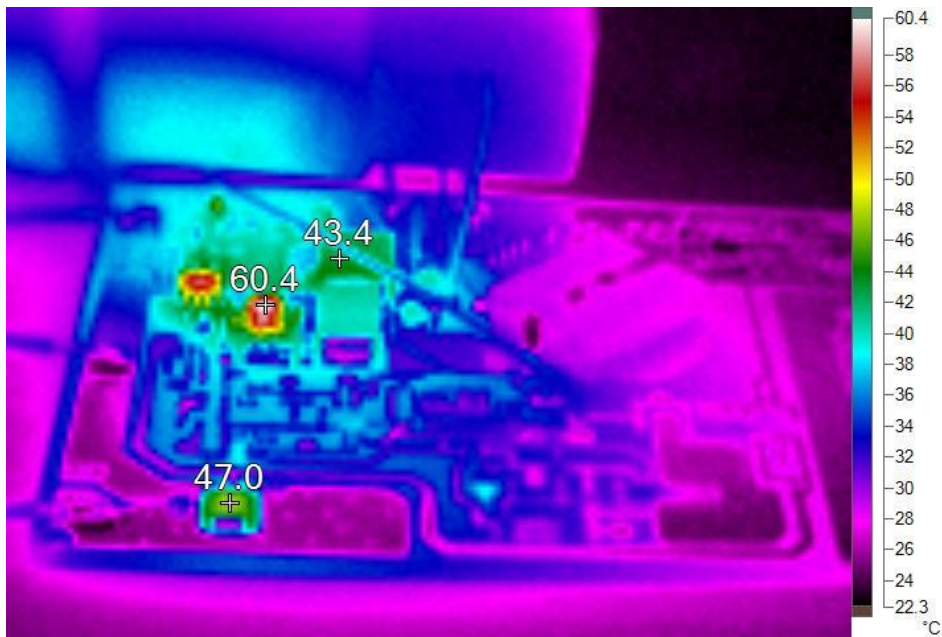
Figure 43. Thermal photo of the ZVS-CV converter at full load.
