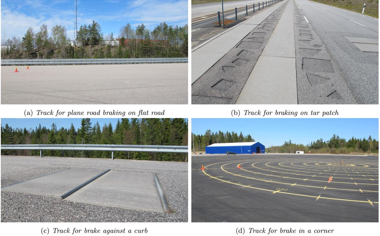
Figure 3.7: *Tracks used for measurements*
