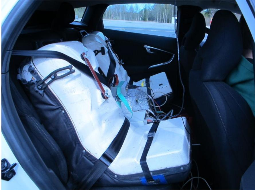
Figure 3.3: *Loading using dummies with weights added inside them, and signal processing equipment between the dummies*
