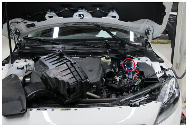
(b) *Measurement ECU mounted in the car*
