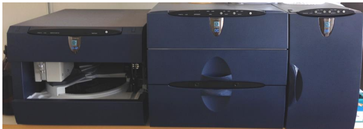
Figure 6: Dionex ICS-5000 HPLC system, equipped with CarboPac PA1 columns.
