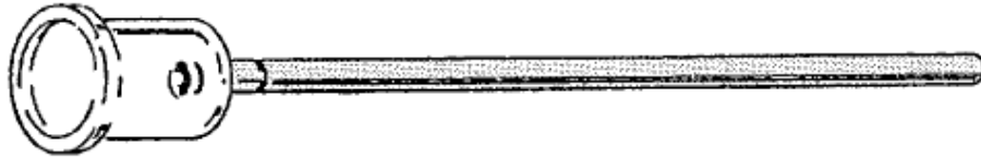
Figure 9: A penetrometer constructed of an insulated glass and a metal stem (Micromeritics 2008).
