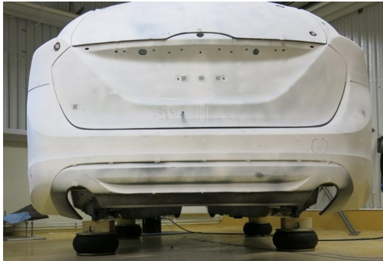
Figure 9: Free-free boundary condition approximation with air-pillows
