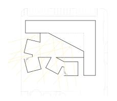
Natural lightening is a very important quality, and to profit even more from the southern exposition the student housing blocks will be cracked and the deep corner of the high massing will be removed.
