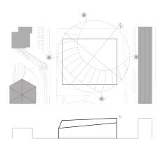
The first factor which determined the massing was the orientation. The top right tip of the site is pointing the northern direction and that is where the highest parts of the building should be located to guarantee a good sun exposition.
