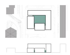
To ensure the harmony between the new building and the existing environment the heights will be adjusted to the surrounding. Lower part facing southern direction will respond to the height of neighbouring Chalmers building and the higher part will have similar height to the housing block.
