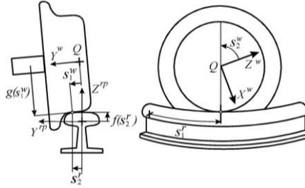
**Fig. 3:** Wheel and rail surface parameters [36].
