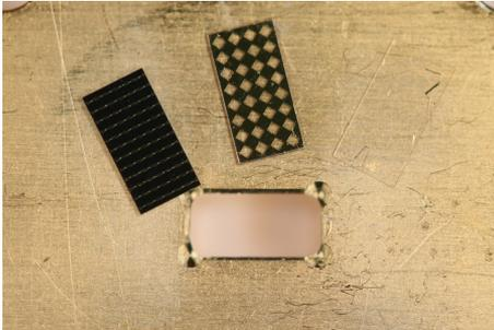
(a) Mounting shim, HBV 2D array, bandpass filter and Quartz matching slab
