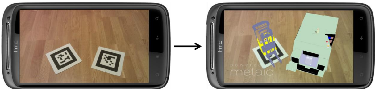
Figure 2-2: Example of AR using frame markers and a smartphone
