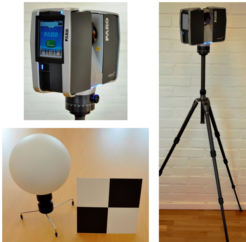
Figure 2-6: In the top left a close-up of the FARO Focus3D 120 phase shift laser scanner, bottom left the reference objects, and to the right the 3D laser scanner mounted on a tripod
