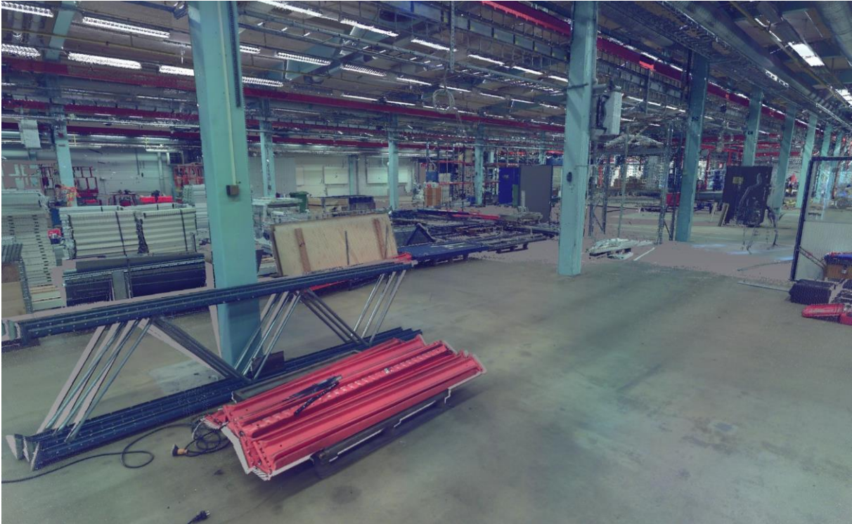
Figure 5-1: The point cloud representing the existing factory building
