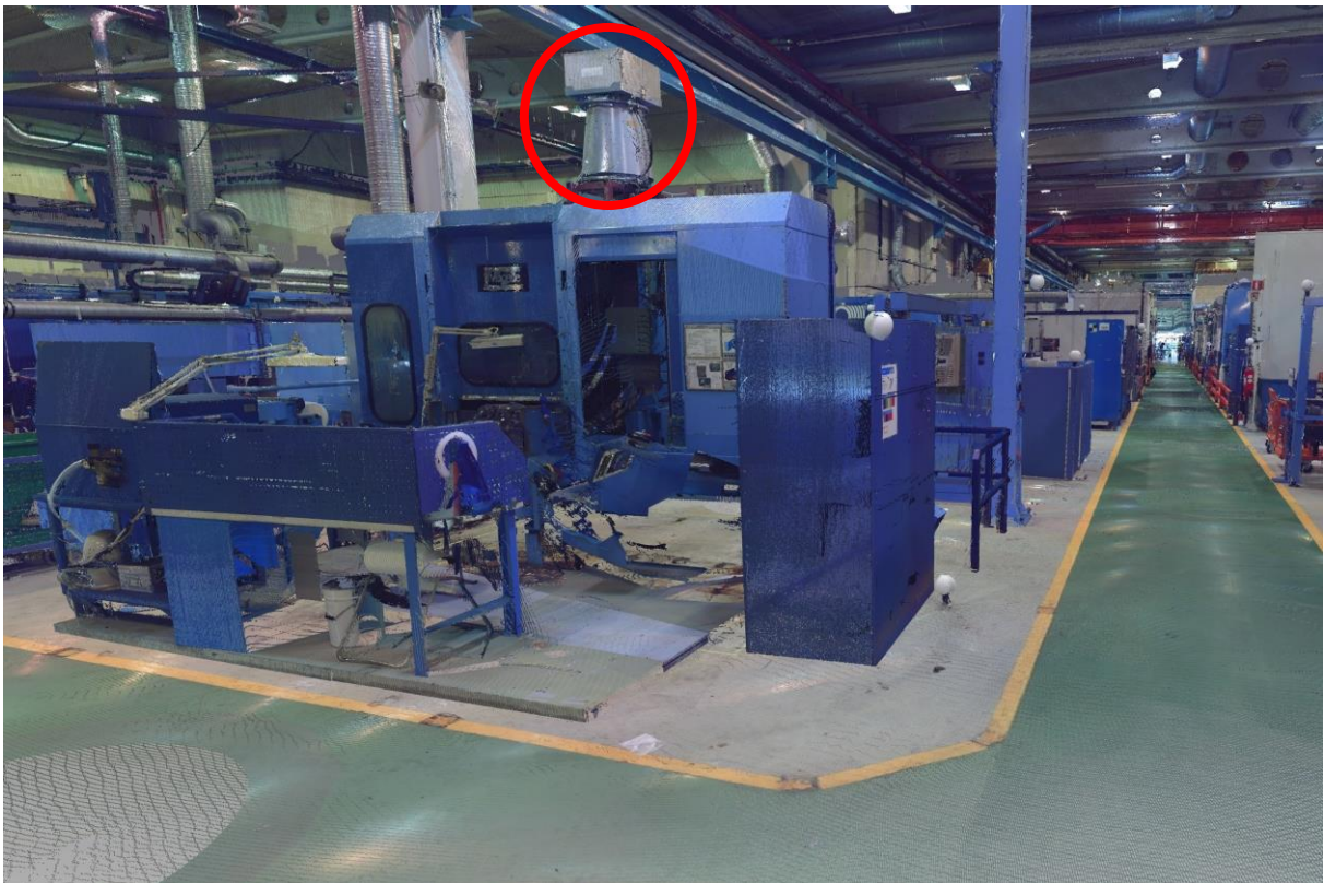
Figure 5-4: The point cloud representing the production system in combination with a section of the point cloud representing the machine (red circle marks the air flue that are missing in the 3D CAD model of Figure 5-3)
