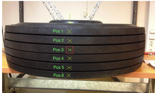
Figure 10: The measured positions of transfer mobility in lateral direction
