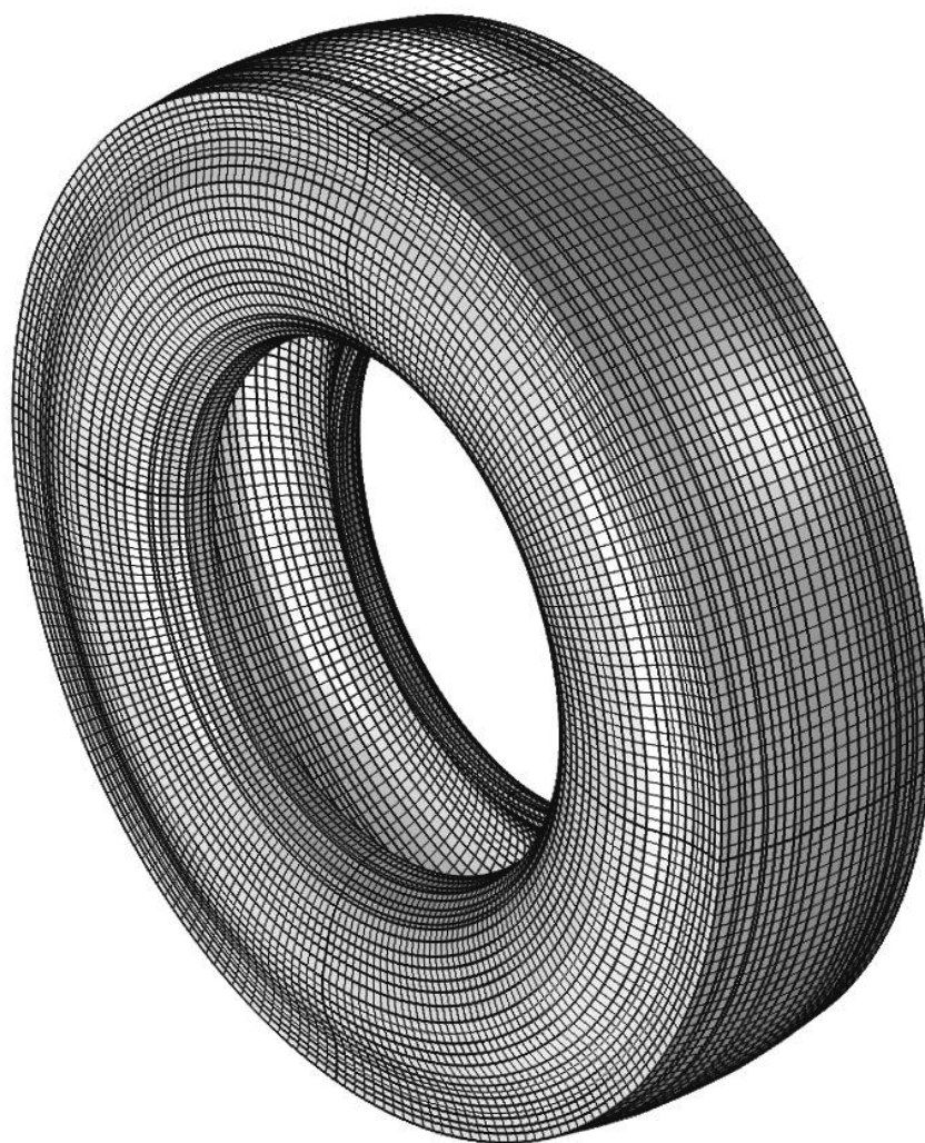
Figure 7: The complete meshed model of the tire.
