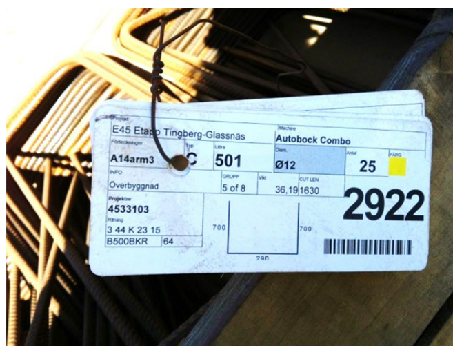
Figure 4.9 Outgoing reinforcement is marked rigorously.
