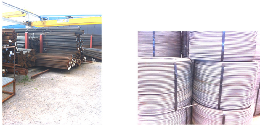
Figure 4.5 Long steel bars (left) and coils (right).
