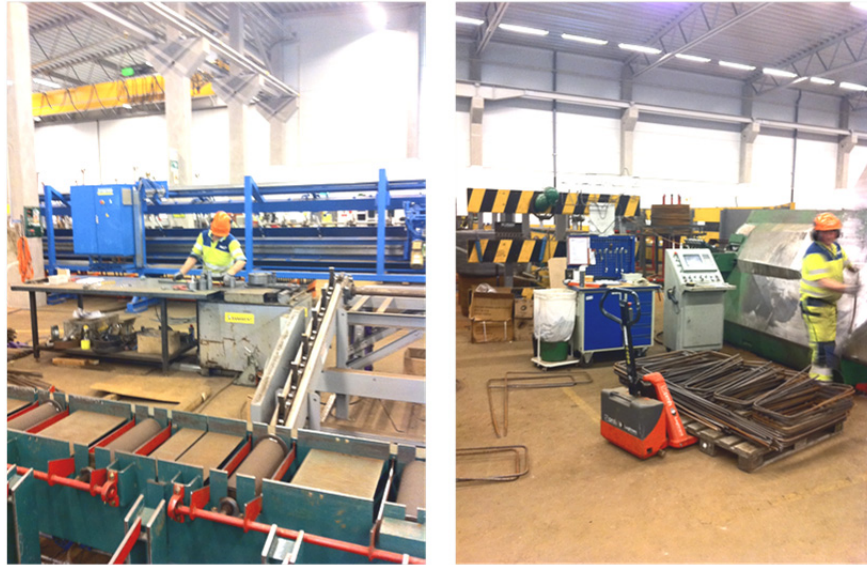
Figure 4.8 Production of CAB in the reinforcement factory.
