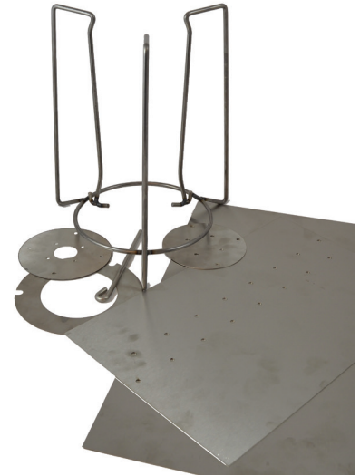
Figure 38. The precut sheet metal parts.
