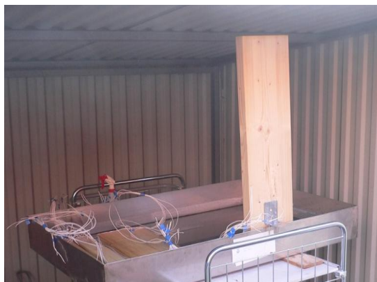
Fig. 9. Sills and vertical stud in the water bath (1–2 mm depth), outdoors under a roof.
