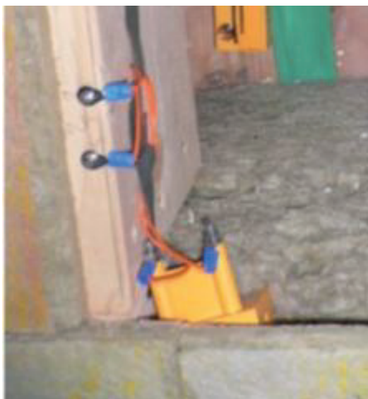
Figure 46. The image shows placement of sensor 16 (RH and temperature) and extension cables for MC bolted onto the outside of the stud.
