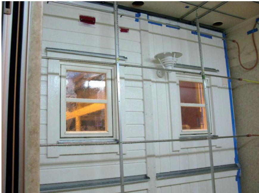
Figure 29. Ongoing testing of two test items, manufacturer B, with horizontal and vertical wood panelling respectively in the rain chamber.
