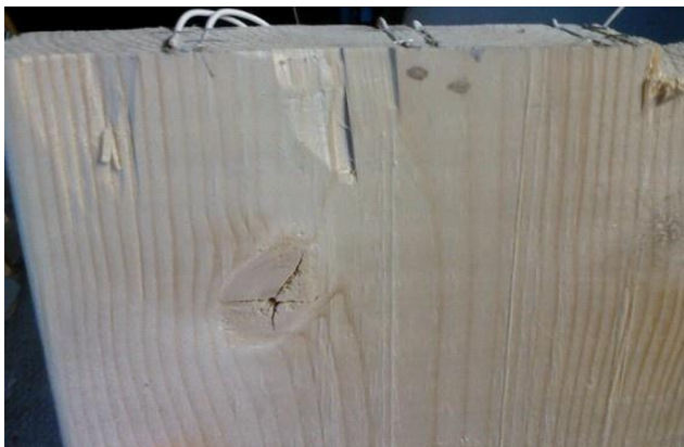
Fig. 23. No visible mould growth on the underside of the sill at the end of the sill. Microbial analysis showed extensive growth.
