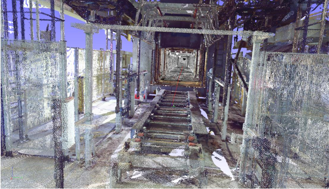
**Figure 6.2:** A view of the entrance of the tunnel through where the object will be moved. The red line shows the path of the object.
