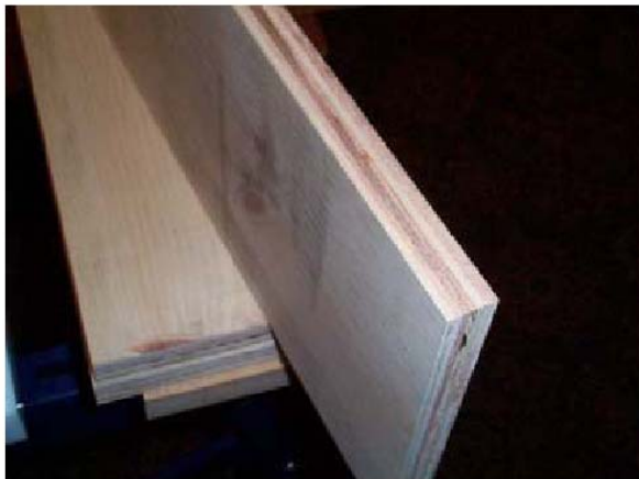
Figure 2.11 Example of a panel in plywood (Piazza, 2004)
