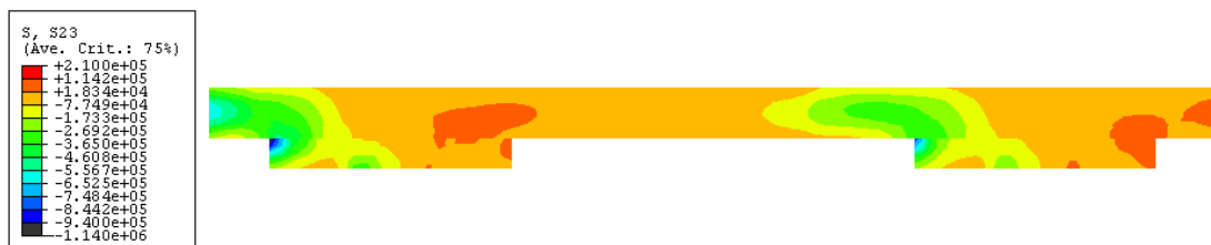
Figure 8.49 Distribution of shear stress \tau_{23} in the Kerto-Q® deck
