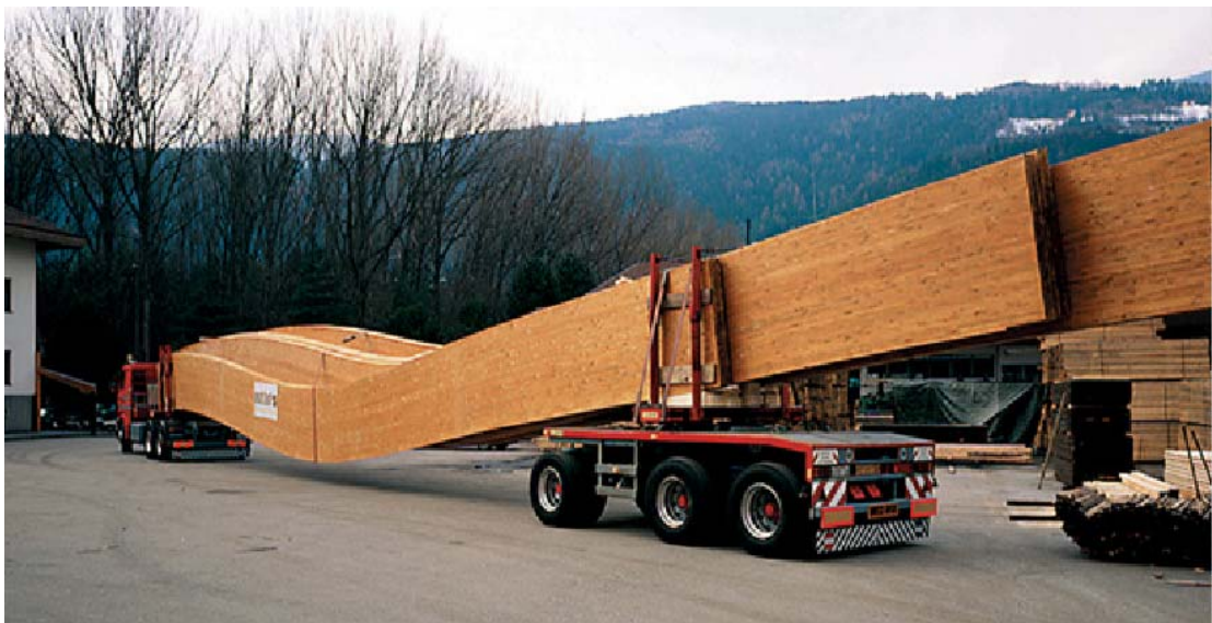
Figure 4.11 Special truck used to transport large timber members (Holzbau Spa)
