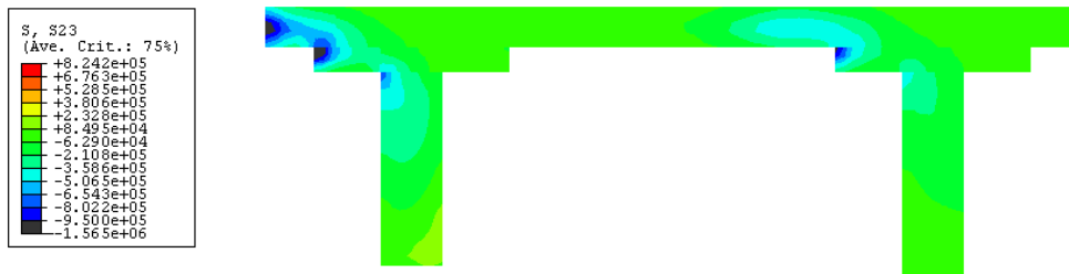
Figure 8.58 Distribution of shear stress \tau_{23} among the cross-section when the wheel is placed over the external unit; the black spots in the Kerto-Q® deck are regions where the value of shear stress is higher than the design value of flatwise shear strength
