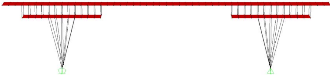
Figure 8.14 Element used to model the bridge, view of the cross-section
