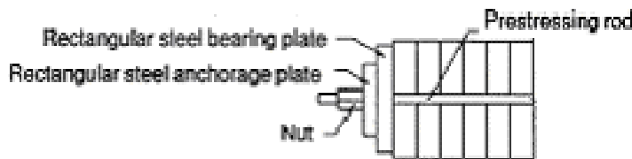
Figure 2.5 Channel bearing plate anchorage configuration. [Ritter (1992)]
