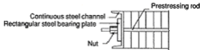
Figure 2.4 Channel bulkhead anchorage configuration. [Ritter (1992)]
