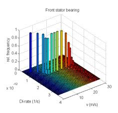
Figure 8: Histogram of damage index rate for front stator bearing at different mean wind speeds.
