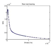
Figure 11: Distribution of total damage rate for rear main bearing.
