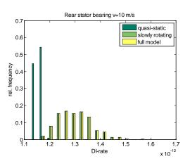
Figure 5: For rear stator bearing, damage rate for mean wind speed 10 m/s, 300 realizations comparison of three drive train model details.
