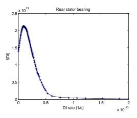
Figure 13: Distribution of total damage rate for rear stator bearing.
