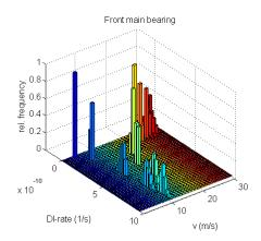
Figure 6: Histogram of damage index rate for front main bearing at different mean wind speeds.
