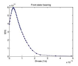
Figure 12: Distribution of total damage rate for front stator bearing.
