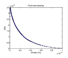
Figure 10: Distribution of total damage rate (Eqn. 5) for front main bearing.
