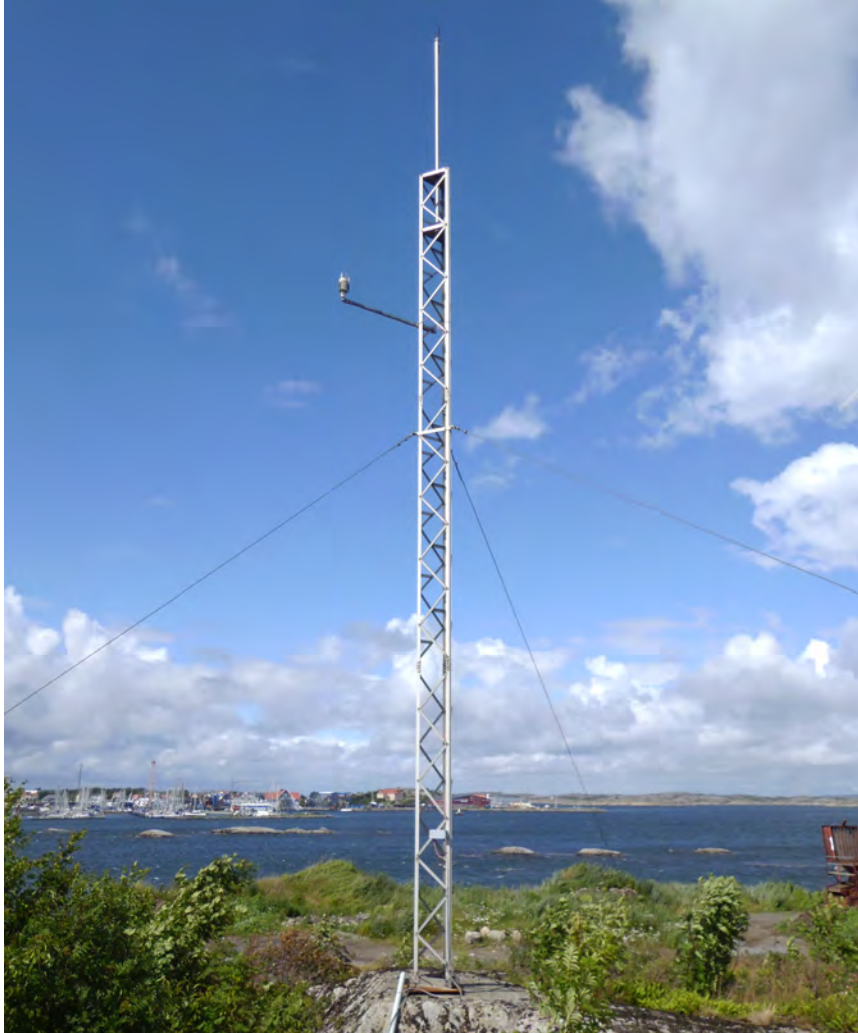
Figure 1.7: Meteorological mast-2, Vaisala weather transmitter at around 9 meters, 3 guy wires that support mast-2 and at the back to left: sea water towards Öckerö and to right sea water towards Björkö and Hisingen
