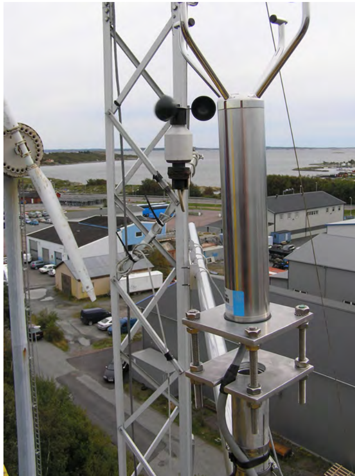
Figure 1.4: WSO and WST on their booms, view from WSO. In the background is Chalmers wind turbine and buildings towards Hönö ferry station
