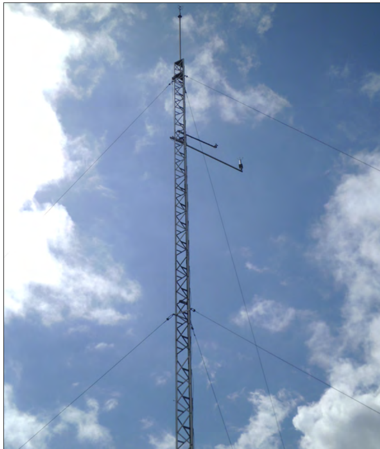
Figure 1.2: Meteorological mast-1, Wind Master on top spar, Wind Observer on a 3 meter boom, Cup anemometer on 1.4 meter boom and also 6 guy wires that support mast-1
