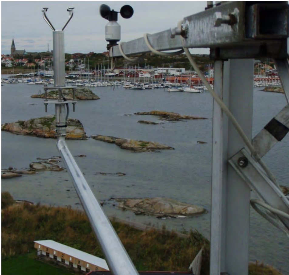
Figure 1.3: WSO and WST on their booms at about 20 m pointing towards Northwest about 318^\circ pointing towards Öckerö community church, Tangential view from the mast-1
