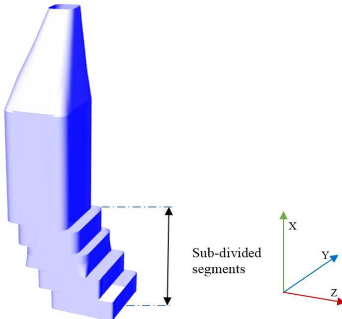
Figure 6.4 Derrick with sub-divided segments in the vertical direction.
