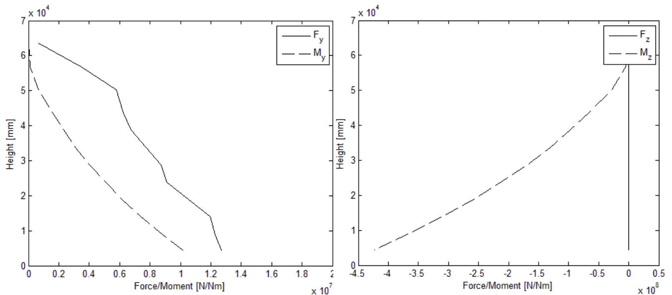
Figure 9.2 Shear force and moment diagram, beam sea.
