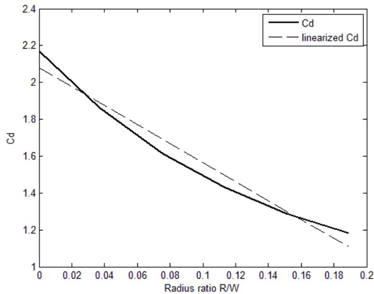
Figure 4.3 Drag coefficient of  $0^\circ$  angle of attack for different corner radii.
