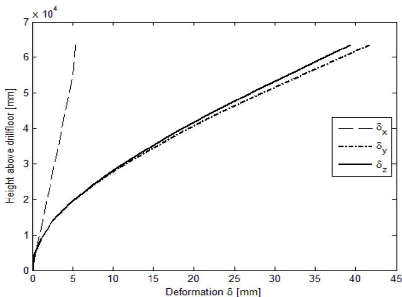
Figure 9.5 Deformation of derrick structure at quart sea.
