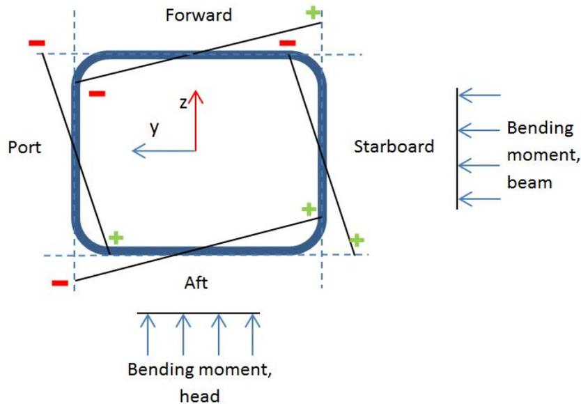
Figure 9.4 Axial stresses on the derrick's outer shell due to the bending moments.
