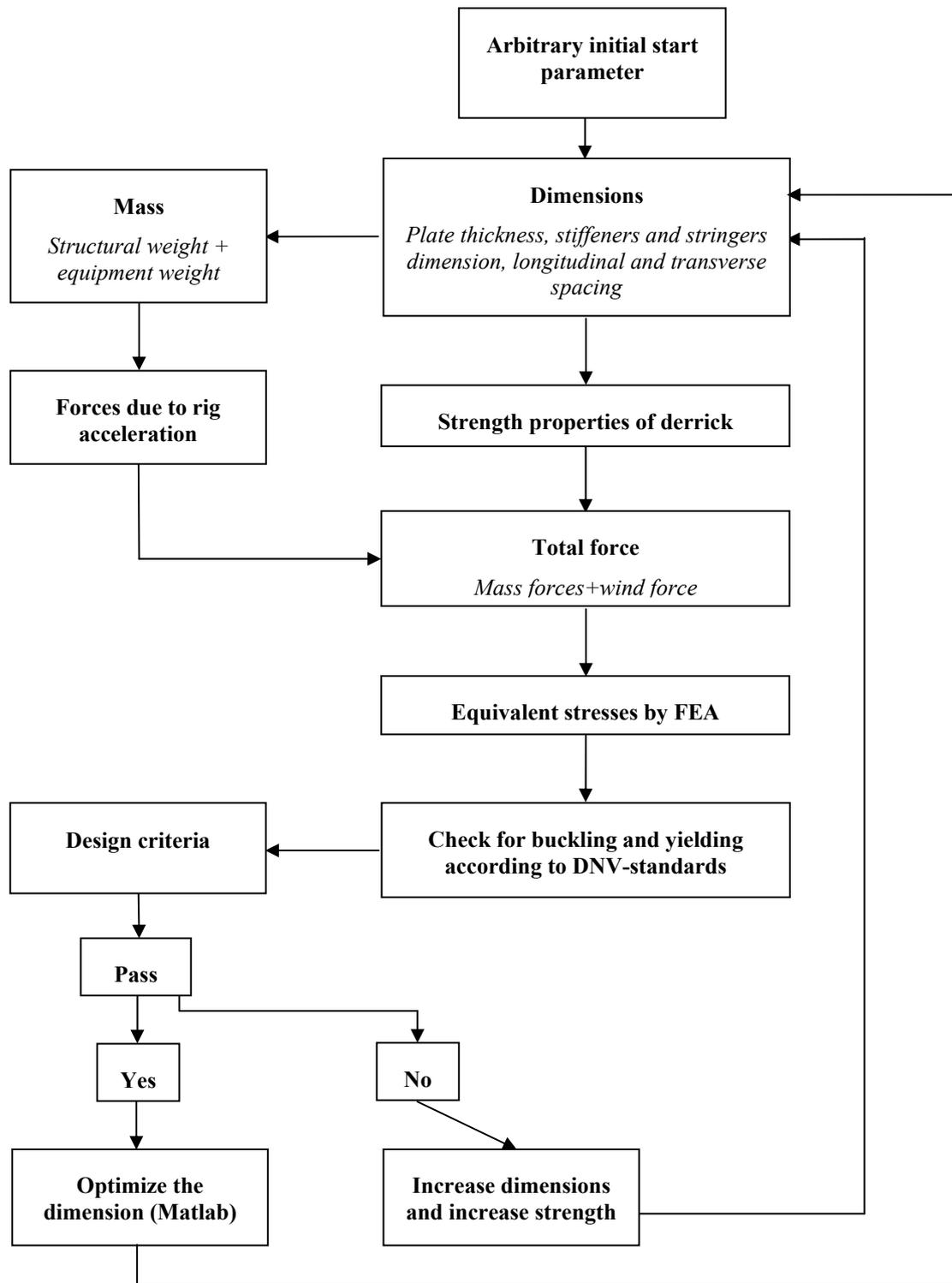
Figure 1.3 Schematic procedure of the methodology in present study.
