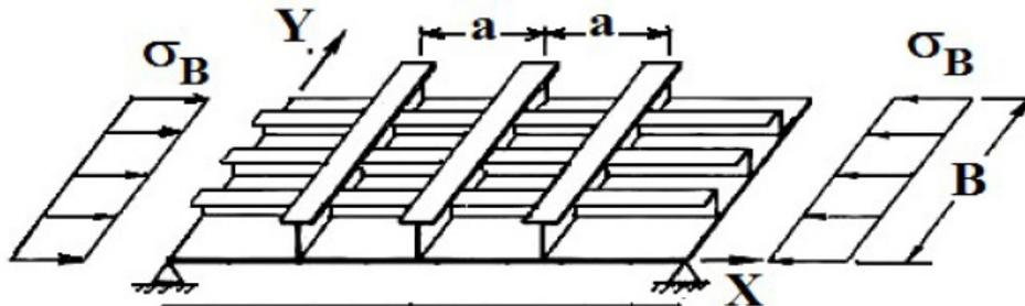
Figure 5.1 Stiffened plate in both the longitudinal and transverse directions under a compressive load.
