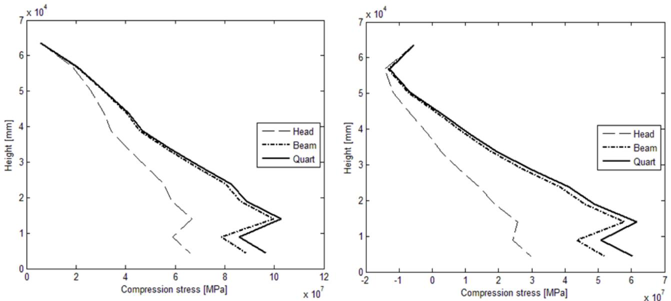
Figure 9.6 Compressive stresses. In the left, corner between port and forward. In the right, corner between starboard and forward.
