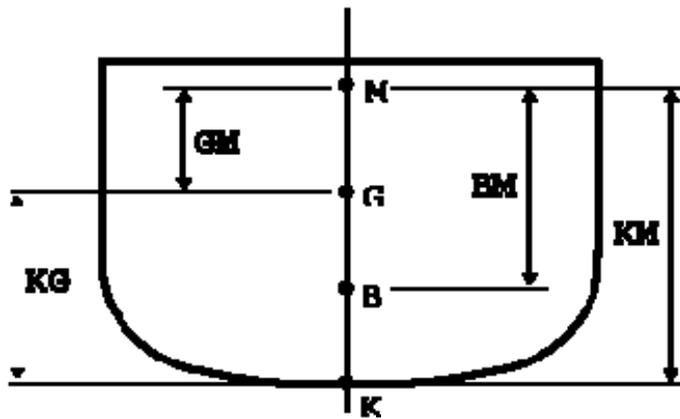
Figure 2.1 Definition of the hydrostatics parameters.
