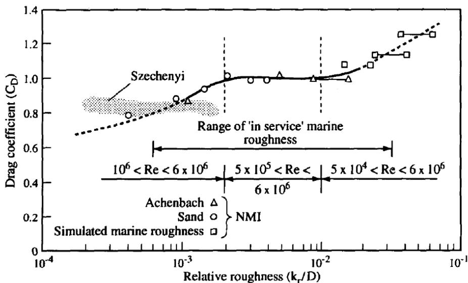
Figure 2.5 Drag coefficient for truss derrick with different surface roughness, from [16].
