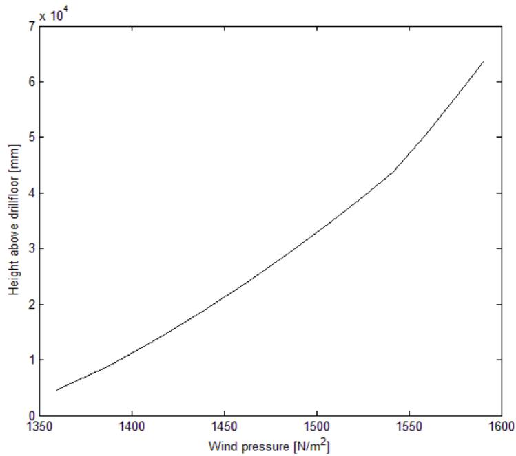
Figure 4.6 Wind pressure along the derrick height.
