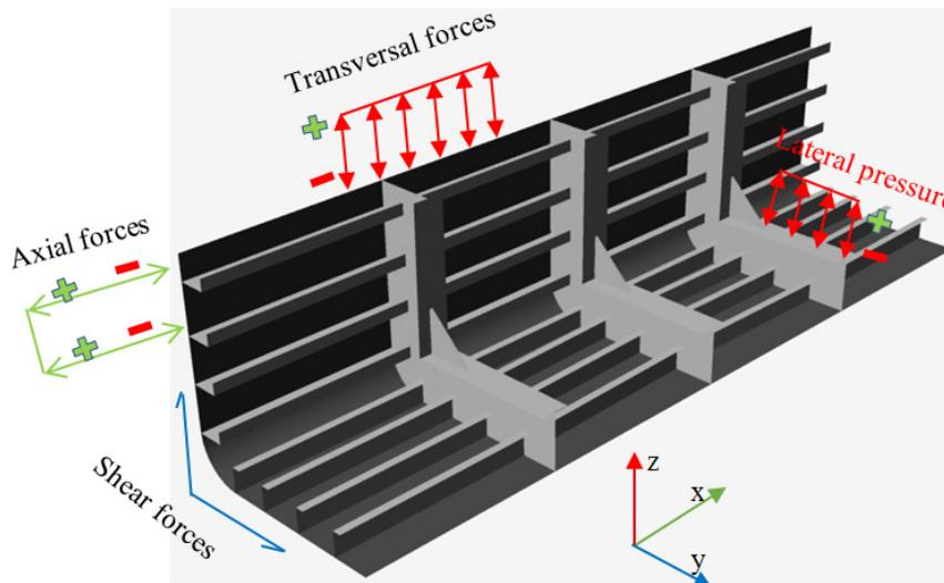
Figure 7.3 Visualization of the stresses for analysis of buckling and yielding.
