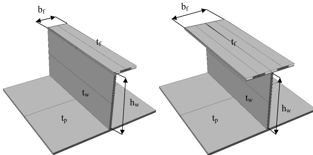
Figure 6.2 L-stiffener and T-stringer used in stressed skin derrick design.
