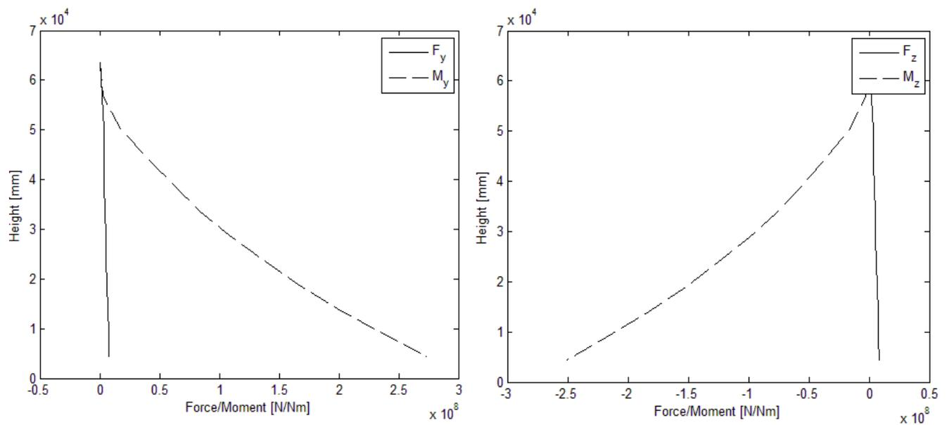
Figure 9.3 Shear force and moment diagram, quart sea.
