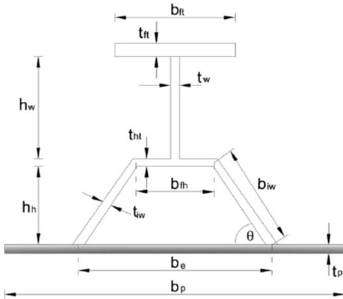
Figure 6.3 Y-shaped beam, from [28].
