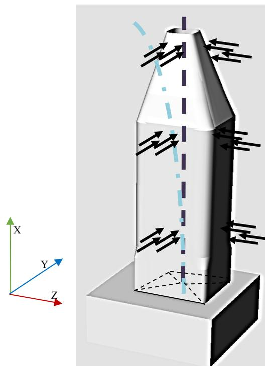
Figure 7.1 *Stress-deformation analysis of a stressed skin derrick utilizes the beam theory with deflection. The arrows represent the wind force acting on the derrick.*
