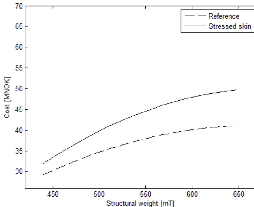
Figure 9.7 Manufacturing cost of reference derrick and stressed skin derrick.
