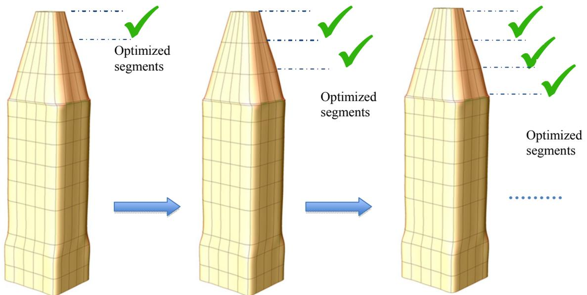
*Figure 8.6 The optimization restricts variable parameters to only the current ones at each segment in order not to involve too many variables at the same time. This keeps the optimization time at its lowest possible.*
