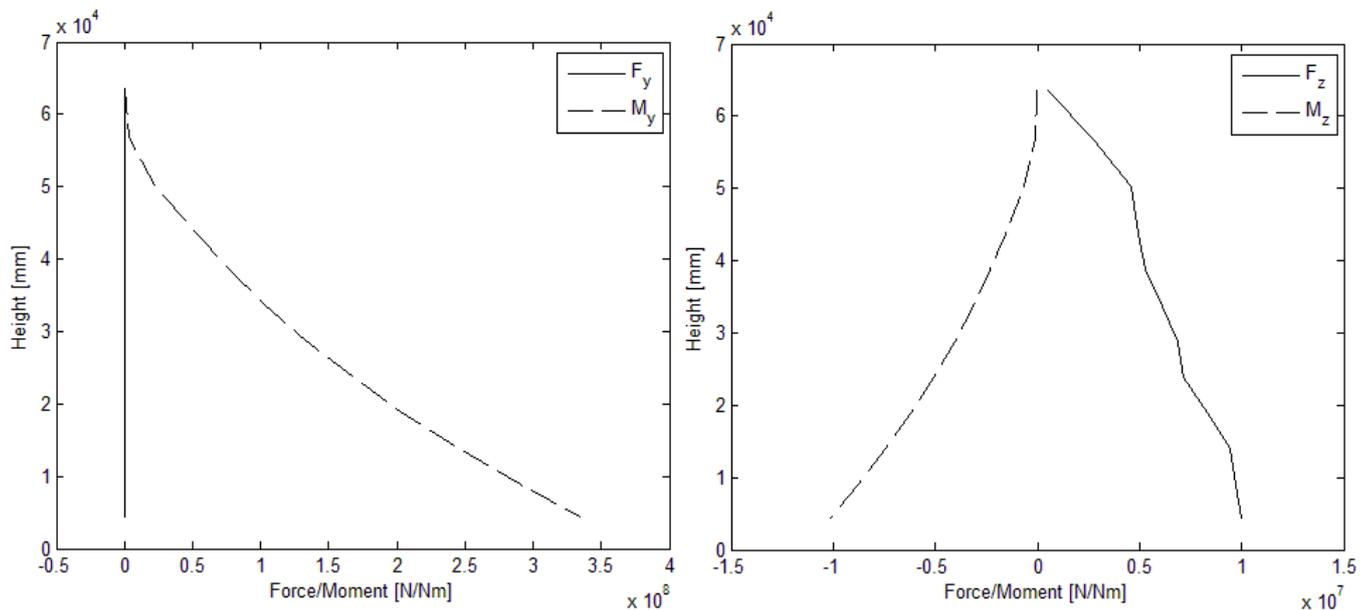
Figure 9.1 Shear force and bending moment diagram, head sea.
