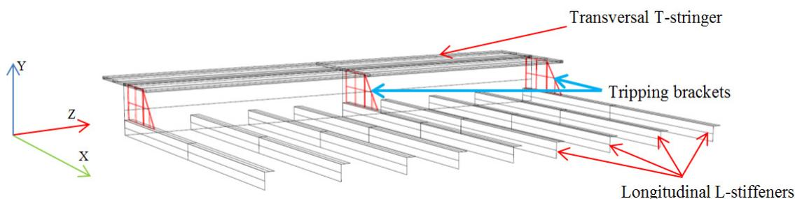
Figure 6.6 Stringer and stiffener with supported tripping brackets in every fourth stiffener indicated with red colour.
