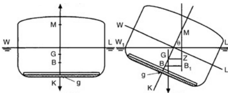
Figure 2.2 Ship in a heeling condition.
