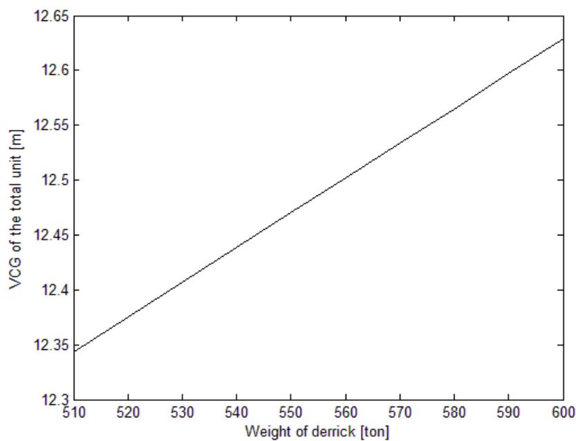
Figure 2.3 Derrick weight influence on the vertical centre of gravity.
