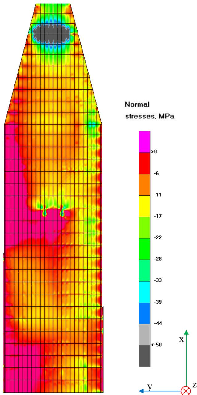
Figure B.1 Stresses in the transverse direction, starboard from [15].
