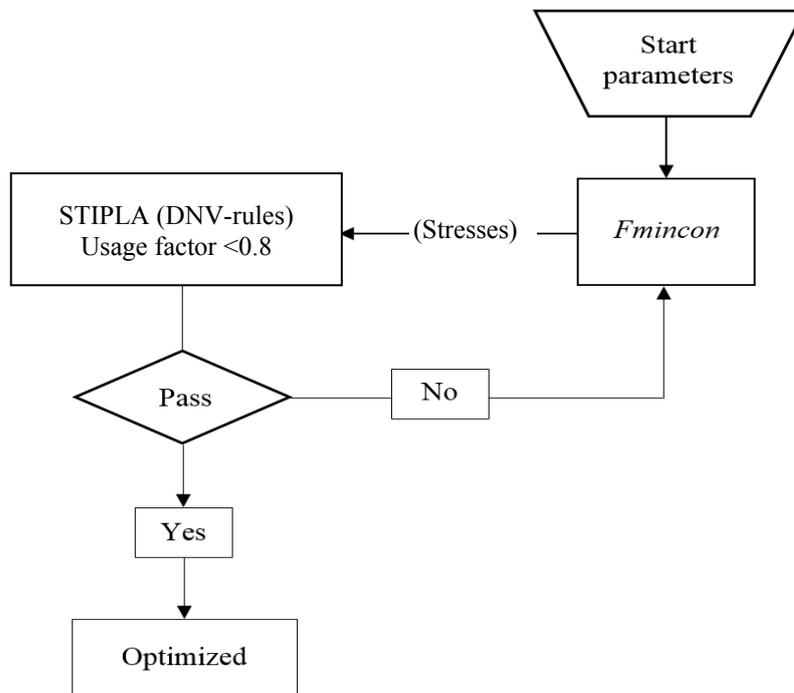
Figure 8.3 Schematic optimization methodology.
