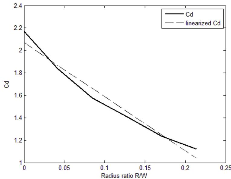
Figure 4.5 Drag coefficient of 90° angle of attack for different corner radii.
