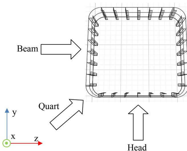
Figure 4.1 Top view of cross section; wind loads in three different study cases.
