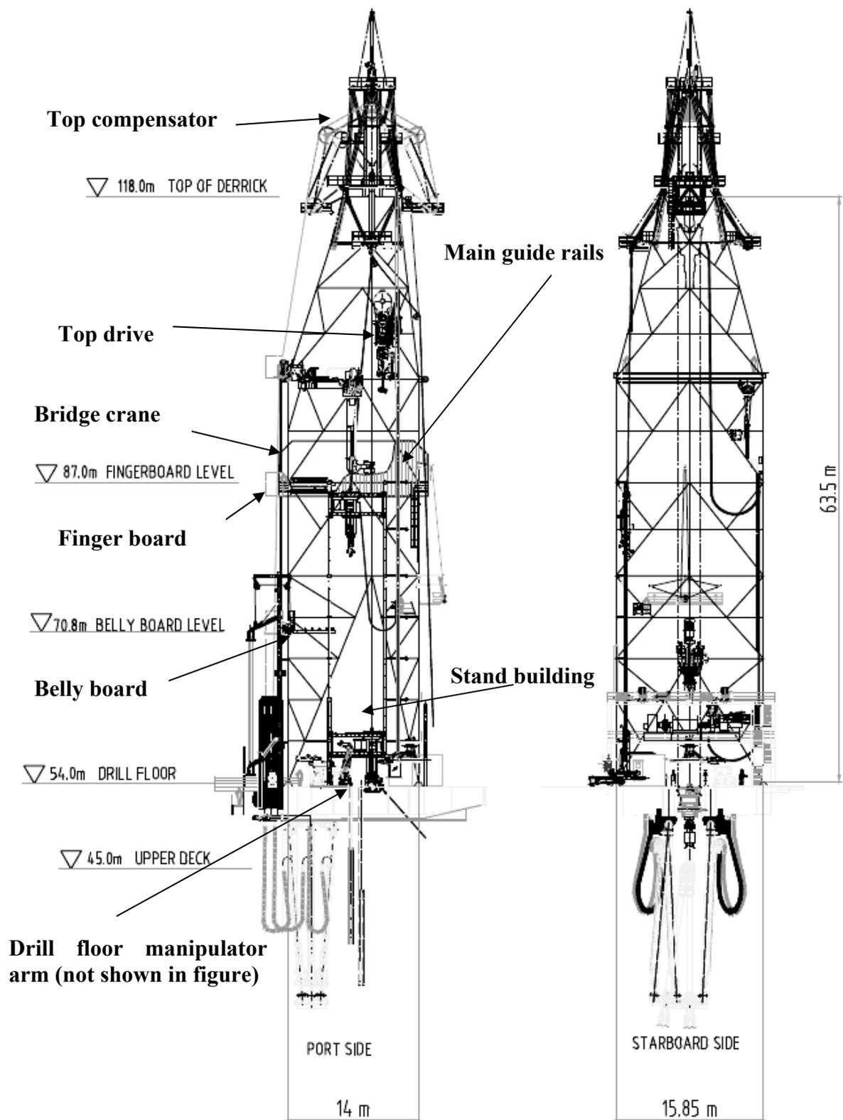
Figure 3.1 Reference derrick with dimensions and heaviest equipment.
