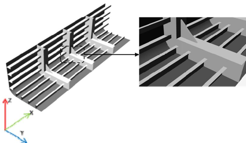
Figure 6.5 Part of the derrick structure utilizing the structural elements used in the proposed design inside the derrick with brackets on right.
