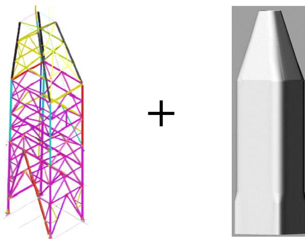
*Figure 1.2 Today's solution of derrick structure for a cold environment. At left, a reference derrick and at right, a protective shell plate.*
