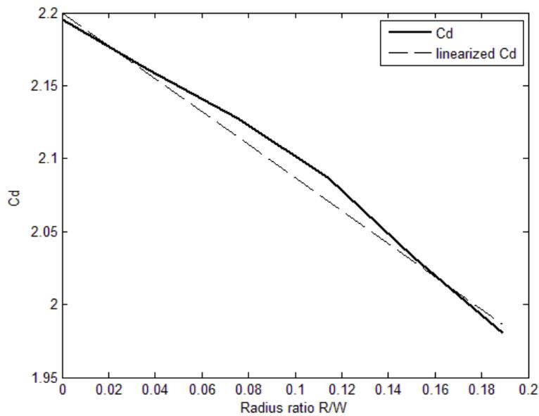
Figure 4.4 Drag coefficient of 45° angle of attack for different corner radii.
