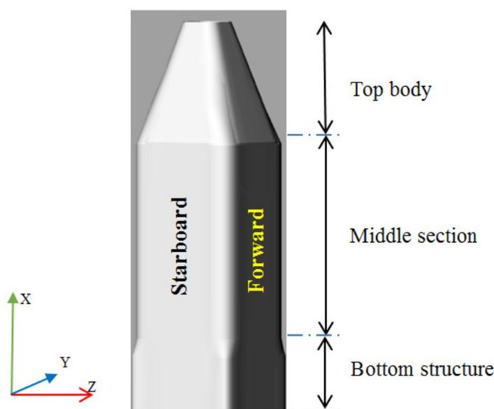
Figure 6.1 Stressed skin derrick with coordinate system in the study.
