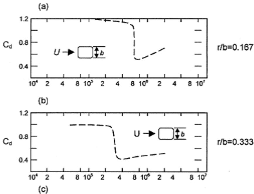
Figure 4.2 Decreasing drag coefficient with an increasing Reynolds number for two different radius ratios, from [19].
