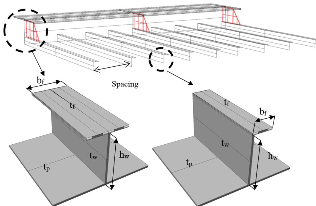
Figure 8.4 Variable parameters during the optimization process.
