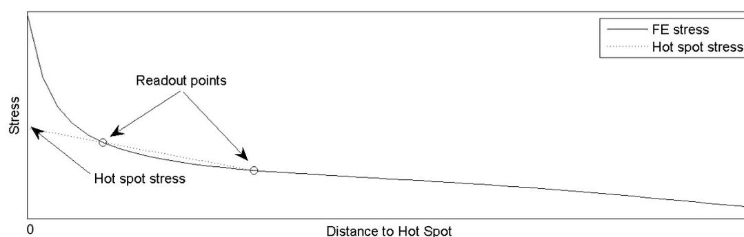
Figure 2.8 Schematic of extrapolation of hot spot stress.
