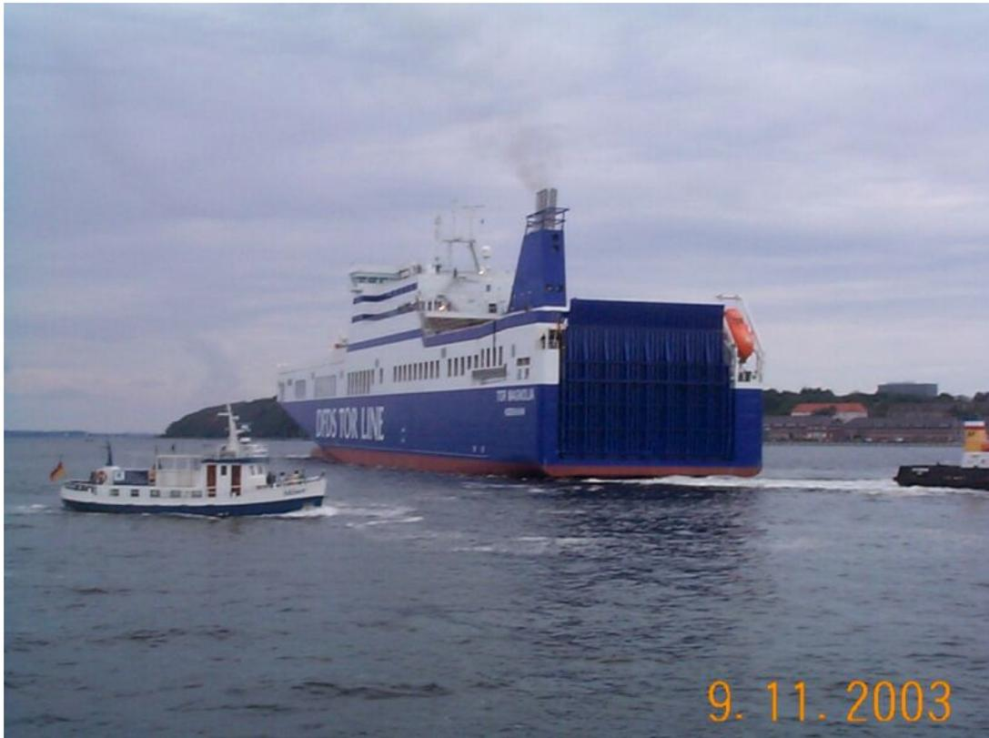
Figure A1 Photo of a straight stern ramp.
