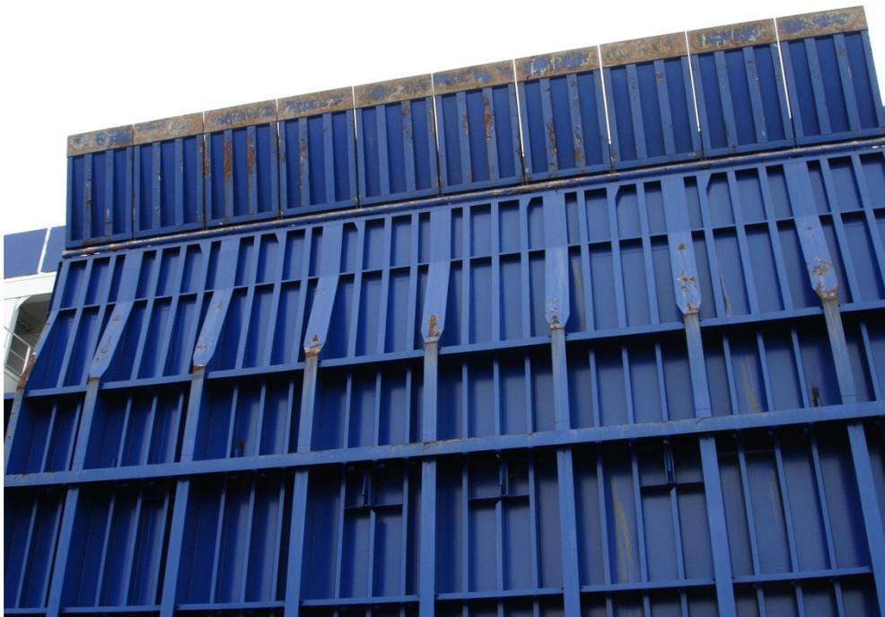
Figure A2 Photo of a straight stern ramp.
