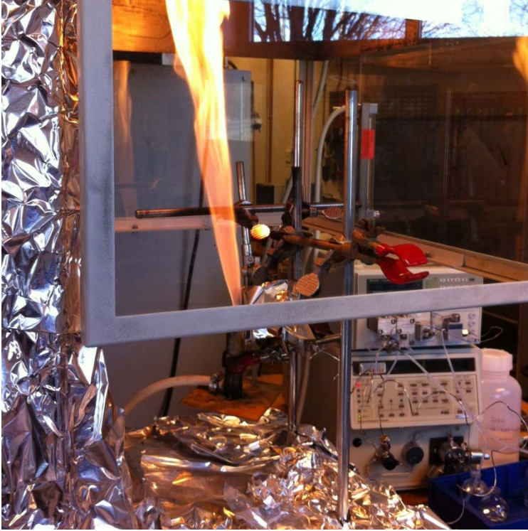
Figure 39 Example of flame when electrolyte and salt is injected, test 25
