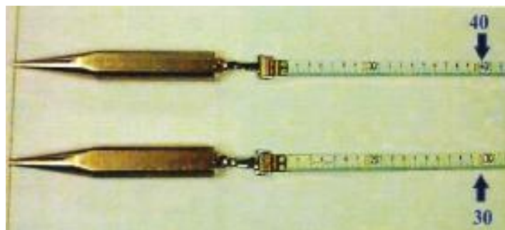
Figure 3. Tampered measuring lines (Kamminga, E)
