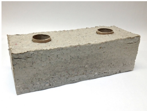
Figure 12: Sigurjónsson, Ásgeir. (2013) A rammed paper brick. A box shape tends to crack at the corners.
