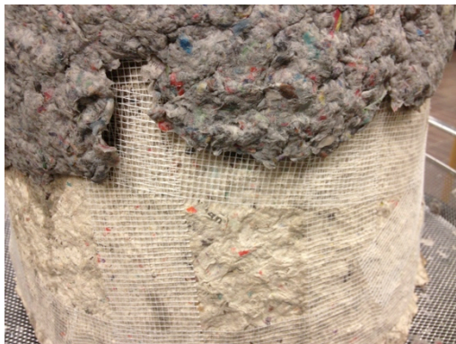
Figure 13: Sigurjónsson, Ásgeir. (2013) Paper daub, reinforced with textile net
