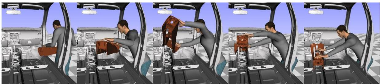
Figure 1: Shows an assembly case where a tunnel bracket is placed inside a car.
