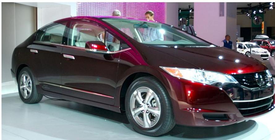
**Figure 2.1:** The Honda FCX Clarity is a limited production car running on Hydrogen, using a fuel cell and an electric motor. From [10].
