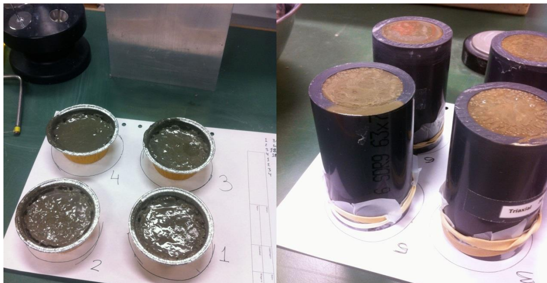
Figure 12 Photo showing the tests of the grout in both cups (left) and cylindrical tubes (right).
