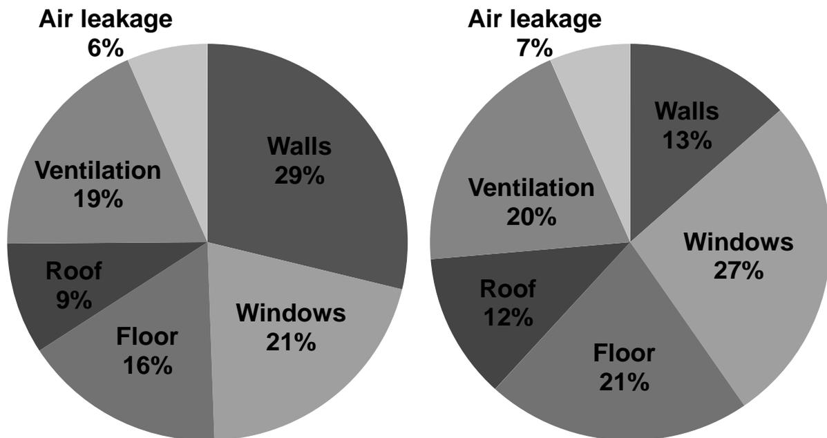
Figure 4.4. Distribution of the heat losses by transmission through the walls, windows, floor and roof, and by the ventilation and air leakages. Left: before the retrofitting. Right: After the retrofitting.
