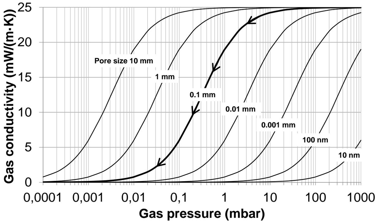
Figure 2.4. Heat transfer by gas conduction in porous materials depending on pore size and gas pressure up to atmospheric pressure at 1 000 mbar. Fumed silica, which is a material used in the VIP core, has pores in the range of 10-100 nm (Based on Simmler et al., 2005).
