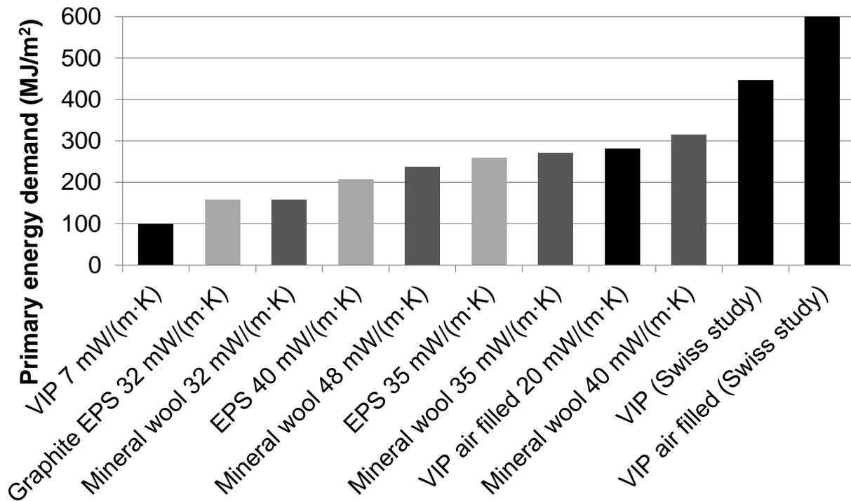
Figure 2.3. Primary energy demand for production of one  $m^2$  insulation material with the same thermal resistance as 25 mm VIPs with a thermal conductivity of 7 mW/(m·K). The values represent average values for a range of products with similar thermal conductivity. The environmental product declarations were made by Institut Bauen und Umwelt e.V. (IBU) (n.d.) in all cases except for the two Swiss VIP calculations which were made by Schonhardt *et al.* (2003).
