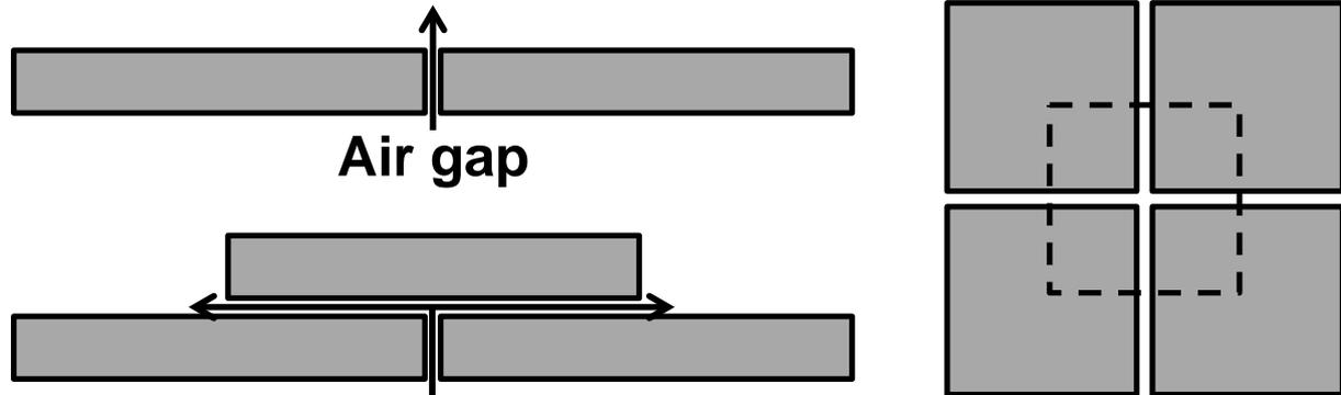
Figure 2.7. Thermal bridge around the perimeter of a VIP. The thermal bridge can be reduced by 64-72% by adding a second staggered layer of VIPs (Ghazi Wakili *et al.*, 2011).
