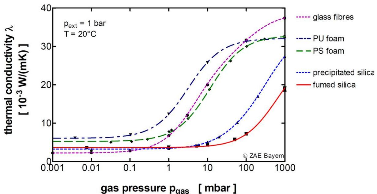
Figure 2.6. Thermal conductivity of different materials which are used in the core of VIPs as a function of the internal gas pressure. Normal atmospheric pressure is 1 000 mbar (Simmler et al., 2005).
