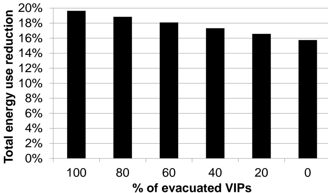
Figure 4.5. Reduction in energy use for different scenarios of the amount of air filled VIPs. The energy use is shown as the reduction of the energy use divided by the energy use before the retrofitting
