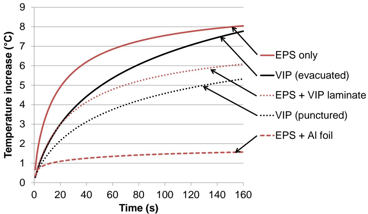
Figure 3.2. Average measured temperature increase in the five setups with a power of 20 mW supplied during 160 s in the 6.4 mm TPS sensor. All materials were measured with 4.7 kPa applied on the upper sample (FIG 3 in Paper II).
