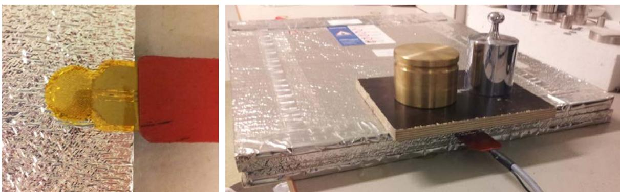
Figure 3.1. Left: TPS sensor on a VIP. Right: measurement setup with the sensor clamped between two VIPs. There was a pressure of 4.7 kPa applied on the upper sample to increase the contact with the sensor. (FIG 1 in Paper II).
