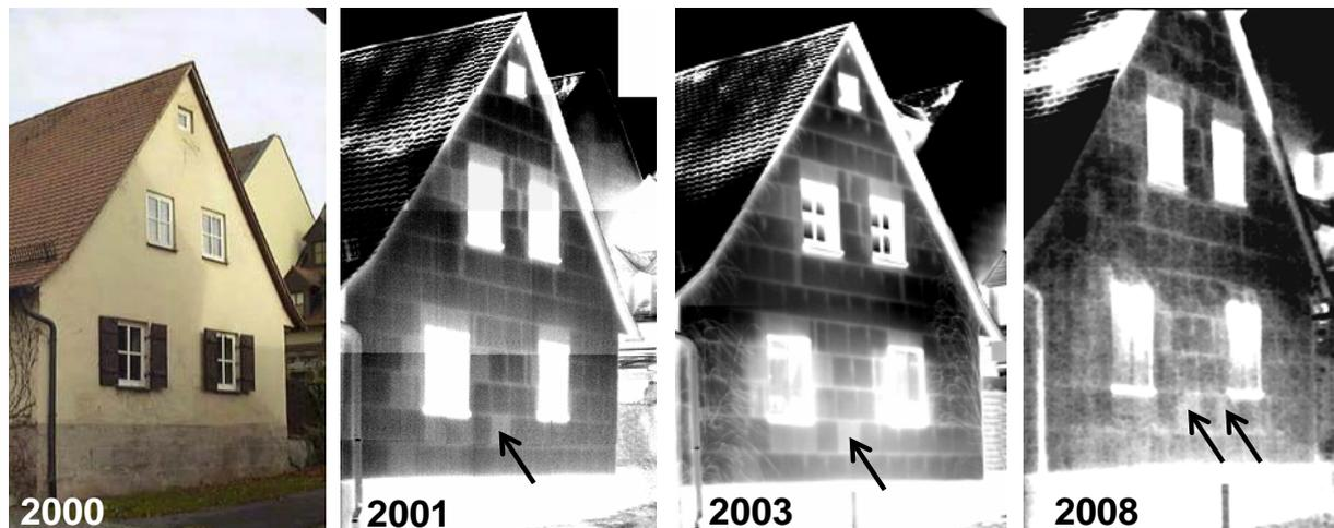
Figure 2.10. The gable of a listed building was retrofitted on the exterior with 15 mm VIPs using a special plastic rail system. The wall was afterwards investigated using thermography. From left: 2000, 2001, 2003 and 2008 (Photo: ZAE Bayern; Heinemann and Kastner (2010)).
