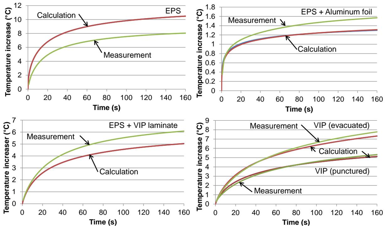
Figure 3.3. TPS measurements compared to the analytical solution for the five setups. Top left: EPS setup. Top right: EPS covered by aluminum foil. Bottom left: EPS covered by VIP laminate. Bottom right: air filled (punctured) and evacuated VIP. (FIG 4 in Paper II).
