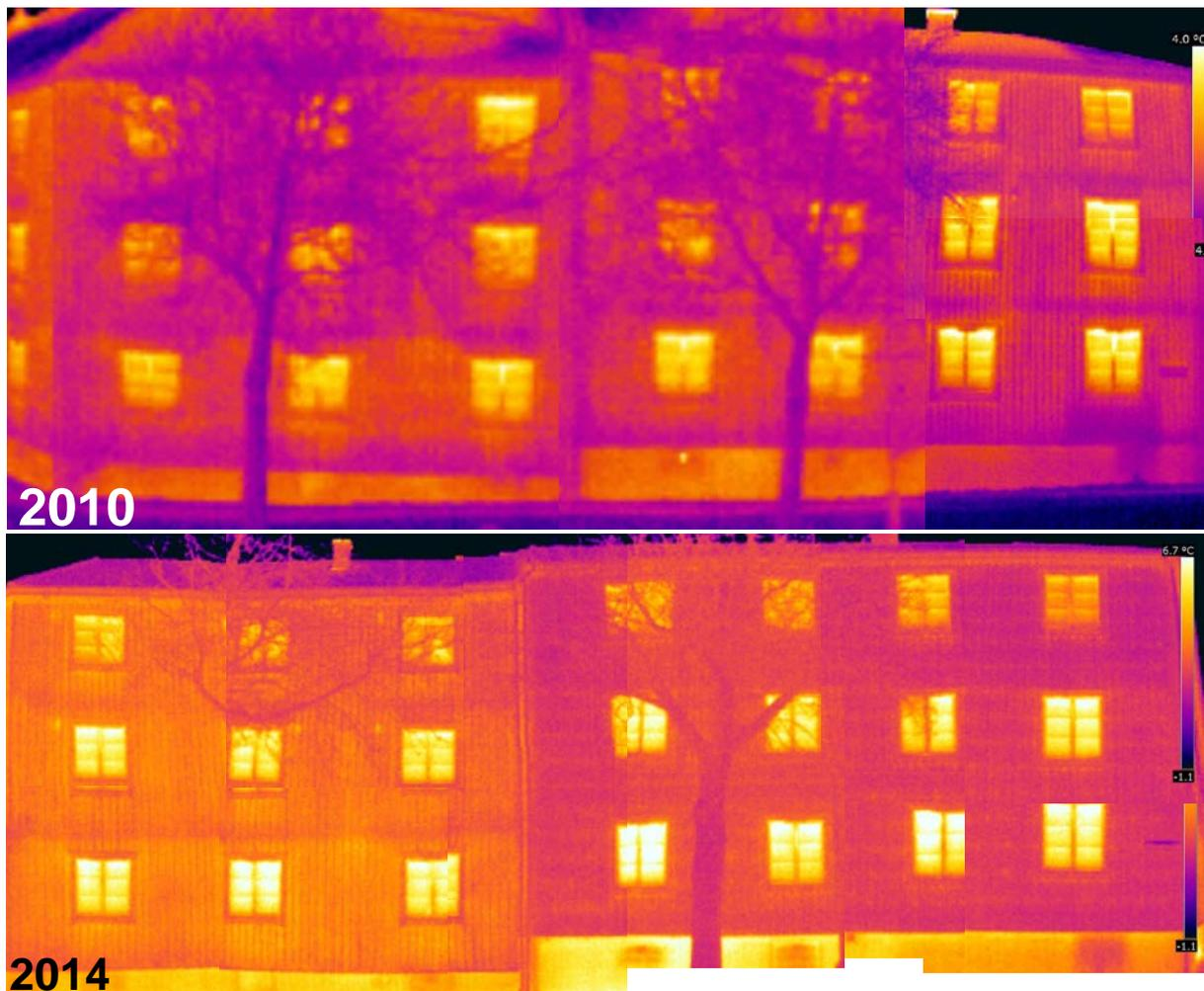
Figure 4.6. Thermograms of the exterior of the wall taken before (top) and after (bottom) the retrofitting. The figure is created by using multiple thermograms. The 12 windows (orange to yellow color) on the right of the wall belong to the retrofitted wall, while the 9 windows on the left of the wall belong to the reference wall.
