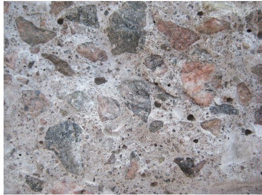
Figure 2.1: Mesoscale structure of concrete. The heterogeneous and random structure of the material is evident and affects the macroscopic material behaviour. The porosity of the cement paste is also observable in this photo.
