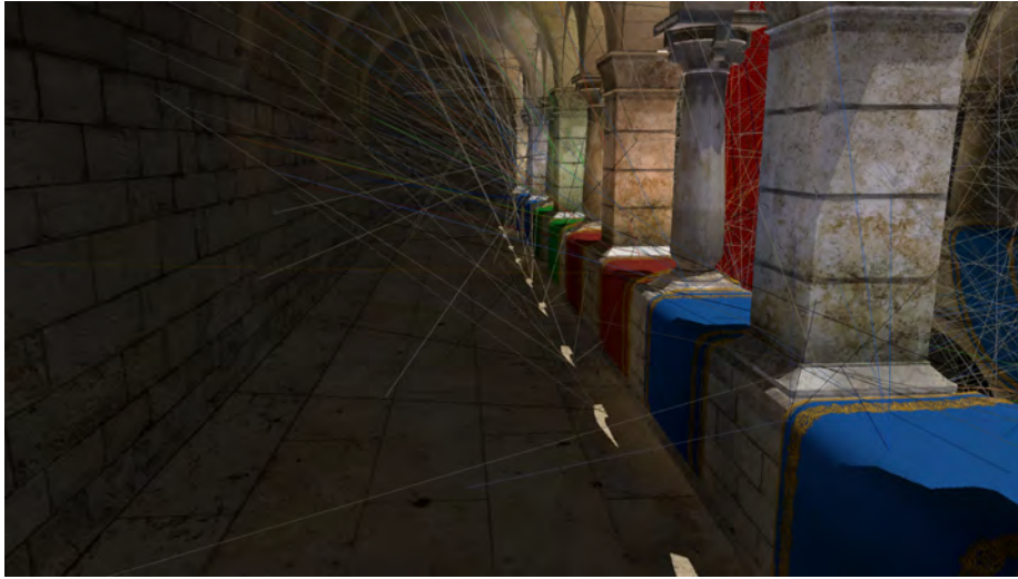
Figure 3.1: Intersection rays are rasterized for demonstration purposes. Note how rays originate from directly lit areas and how each ray's color is determined by the scene material.
