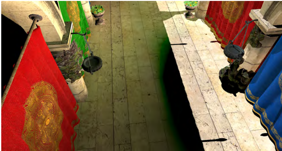
Figure 3.3: Artifacts from using spherical harmonics to store the light in the light volume is visible as large black spots on the floor.
