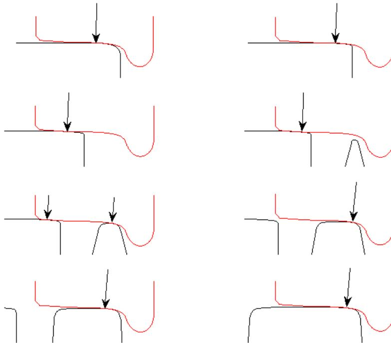
Figure 12. Schematic contact conditions and normal wheel-rail contact forces during a crossing transition
