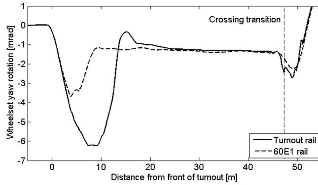
Figure 15. Yaw rotation of leading wheelset (positive yaw in the direction of the curvature). Nominal turnout rail geometry is compared to a fictitious case with a constant 60E1 rail cross-section
