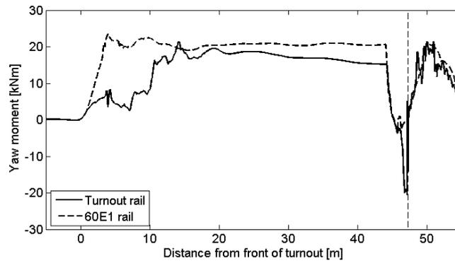
Figure 16. Yaw moment on leading wheelset (positive moment on wheelset in the direction of the curvature). Nominal turnout rail geometry is compared to a fictitious case with constant 60E1 rail cross-section
