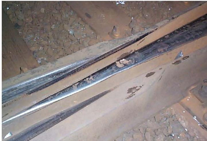
Figure 22. Spalling (loss of material chips) on a manganese steel crossing nose. From [6]
