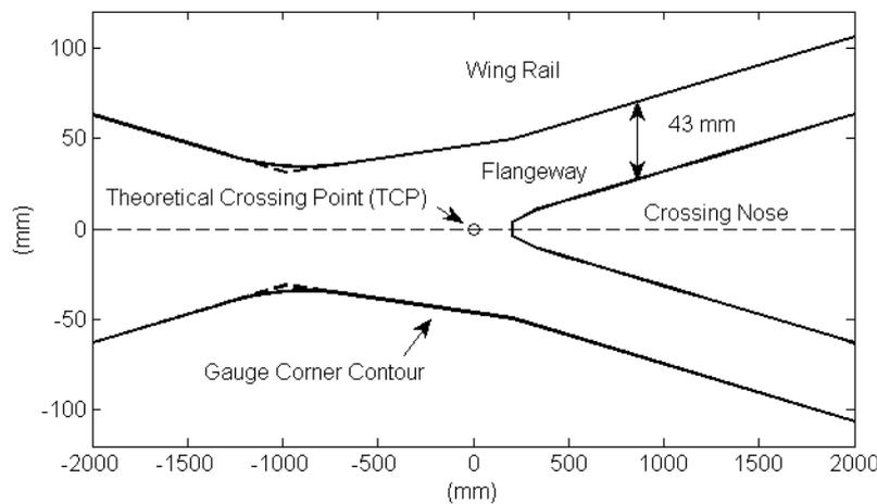
Figure 11. Top view of gauge corner contour at crossing
