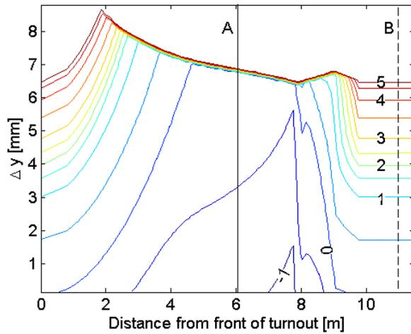
Figure 8. Contour plot of rolling radius difference [mm] as a function of lateral wheelset displacement towards the switch rail and position from the front of the turnout. The plot is based on the rail geometry in Figure 7 and a nominal S1002 wheel profile
