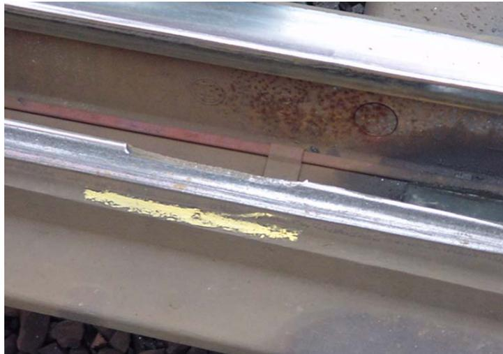
Figure 21. Worn switch rail where a crack has grown from the rail head down into the material, propagated longitudinally and finally turned upwards again causing the removal of a large part of the switch rail. From [6]
