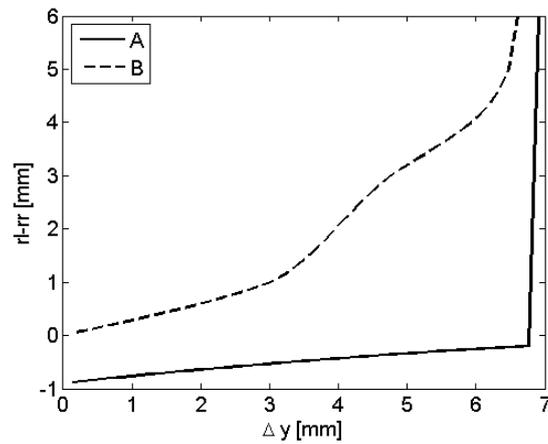
Figure 9 Rolling radius difference characteristics for sections A and B of Figure 8
