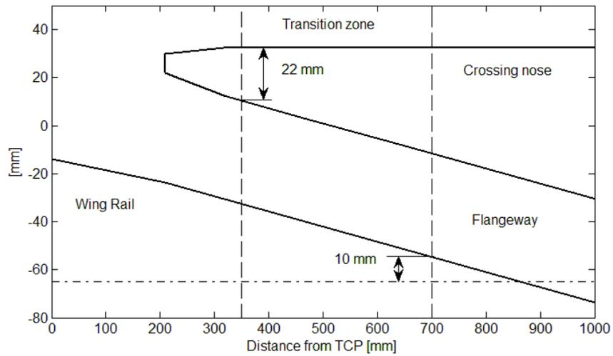
Figure 14. Top view of crossing geometry with crossing angle 1:15. TCP = Theoretical Crossing Point
