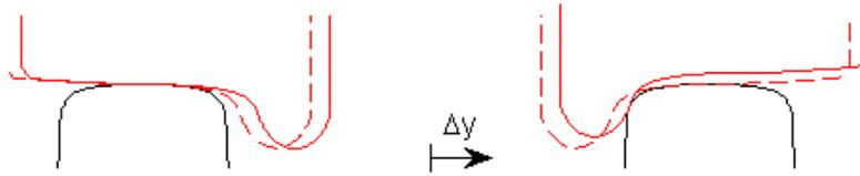
Figure 5. Illustration of vertical wheel movement and change of rolling radius with lateral wheelset displacement  $\Delta y$ . The lateral rail and wheel spacing is not to scale
