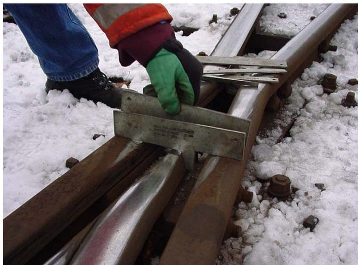
Figure 23. Worn crossing nose as shown by the vertical distance between template and crossing nose. From [6]
