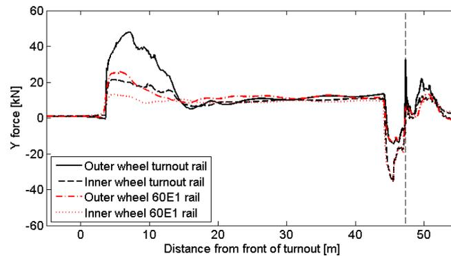
Figure 18. Total lateral wheel–rail contact force acting on inner and outer wheels. Positive force on wheel is directed towards track centre. Nominal turnout rail geometry is compared to a fictitious case with constant 60E1 rail cross-section
