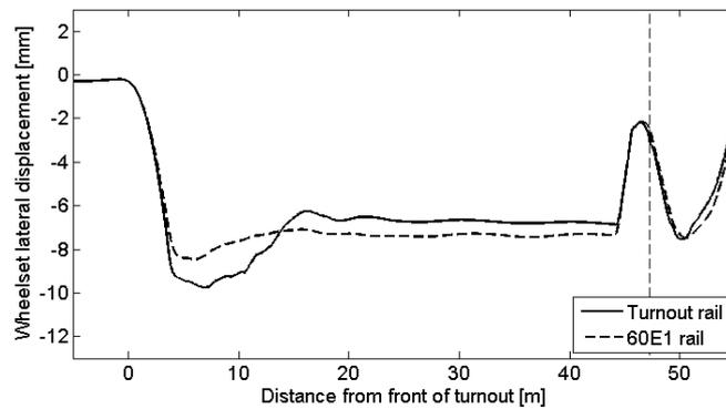
Figure 17. Lateral displacement of leading wheelset (positive towards the inside of the turn). Nominal turnout rail geometry is compared to a fictitious case with a constant 60E1 rail cross-section
