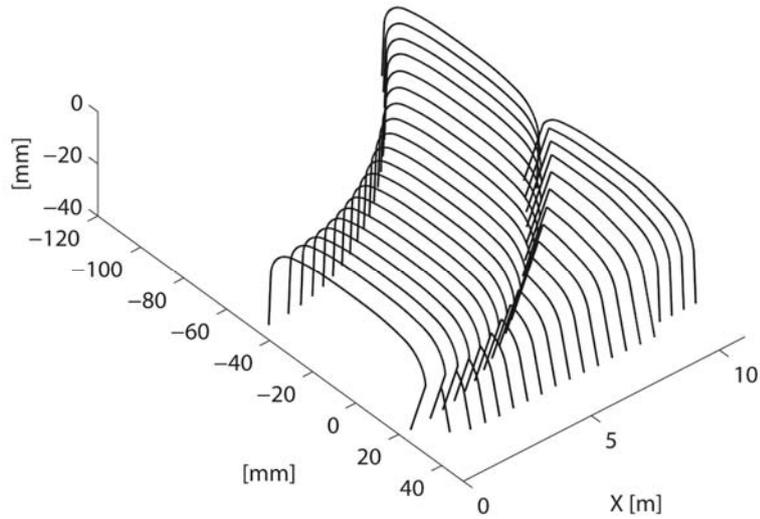
Figure 7. Nominal switch rail sections where X is the distance from the front of the turnout
