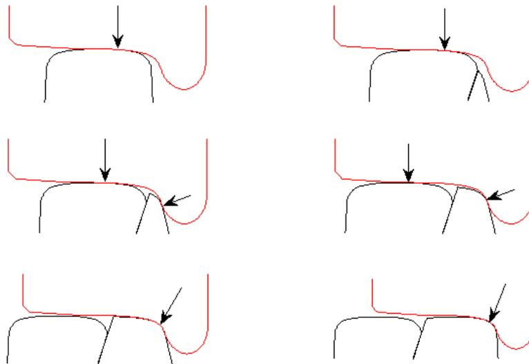
Figure 10. Schematic contact conditions and normal wheel-rail contact forces during a switch transition in the diverging route
