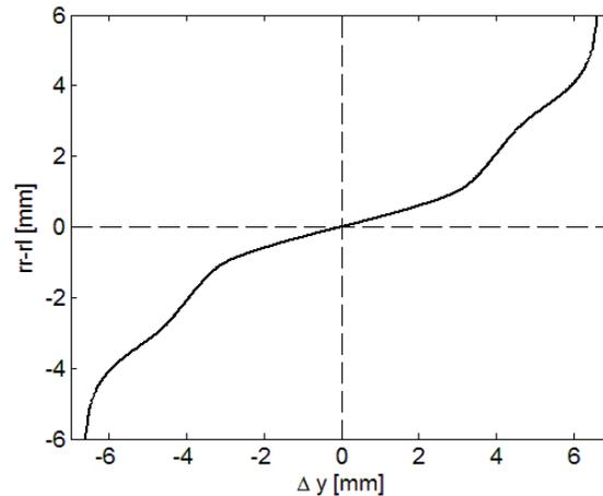
Figure 6. Rolling radius difference as a function of lateral wheelset displacement. Results for a nominal S1002 wheel on nominal 60E1 rails without inclination
