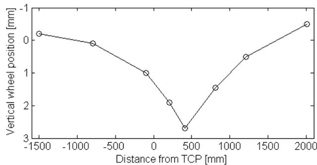
Figure 13. Vertical wheel trajectory, based on vertical wheel positions corresponding to the cross-sections of Figure 13, as a function of distance from the Theoretical Crossing Point (TCP)
