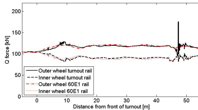
Figure 20. Vertical wheel–rail contact force  $Q$  for the leading wheelset in the facing move of the diverging route
