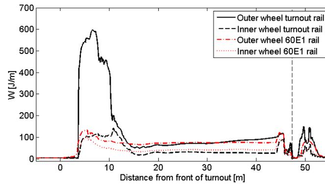
Figure 19.  $W$  (energy dissipation) during a turnout passage for two simulation cases with different rail configurations
