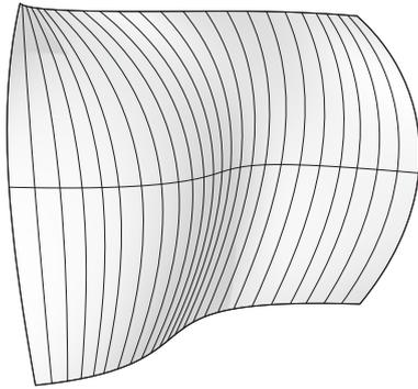
Rebuilt surface through extraction of iso-curves at predetermined densities. Density effects the amount of crumpling
