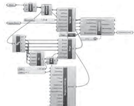
Fig. 125, triangle equalateralisation through the Kangaroo Springs and Hinge forces
