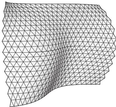
Triangular paneling of rebuilt surface. Panel density is linked to surface iso-curve density
