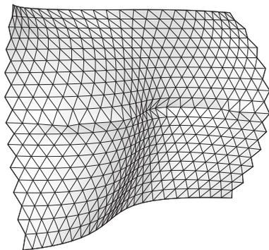
Constraint adjustment at meeting point between floors. Vertex repositioning based on eventual triangle edge length
