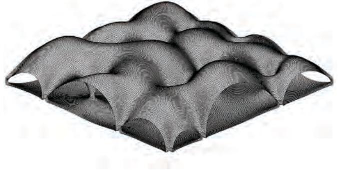
Fig. 45, Kangaroo springs + unary force + anchor points, catenary model generated through Kangaroo (Grasshopper plug-in, Rhino)
