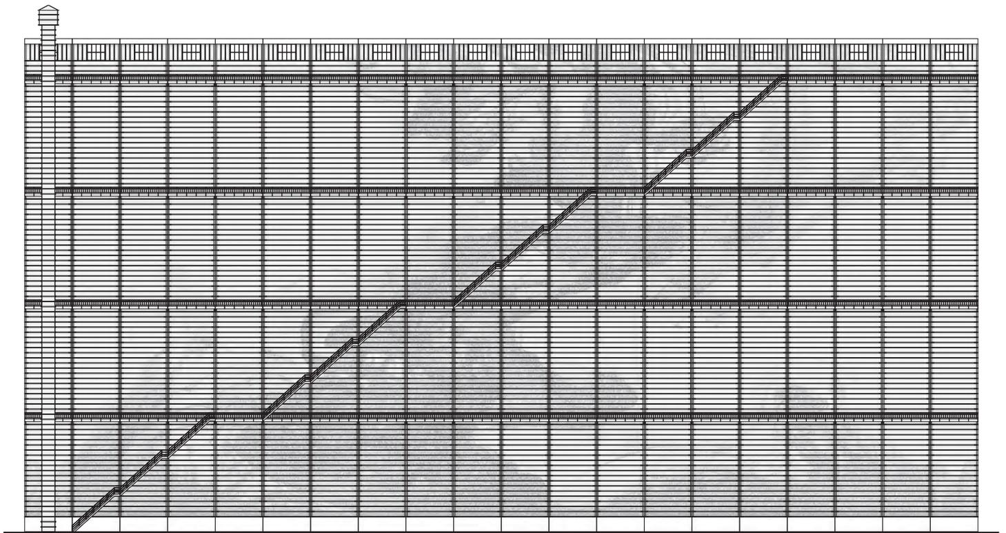
Fig. 132, perforation pattern on unrolled facade 1:800
