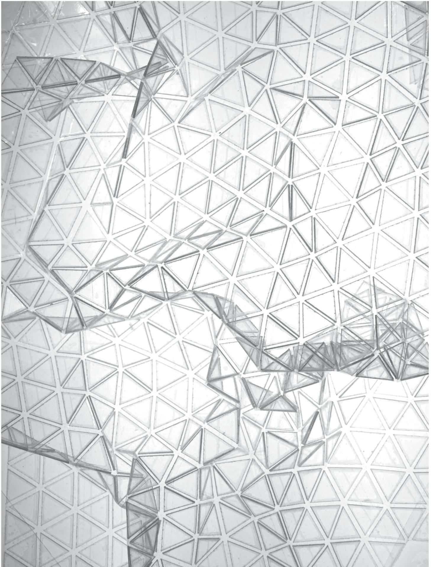
Fig. 113, rationalisation of geological surface: tessellation strategy for surface crumpling. Model: Laser cut polyester triangles on adhesive film
