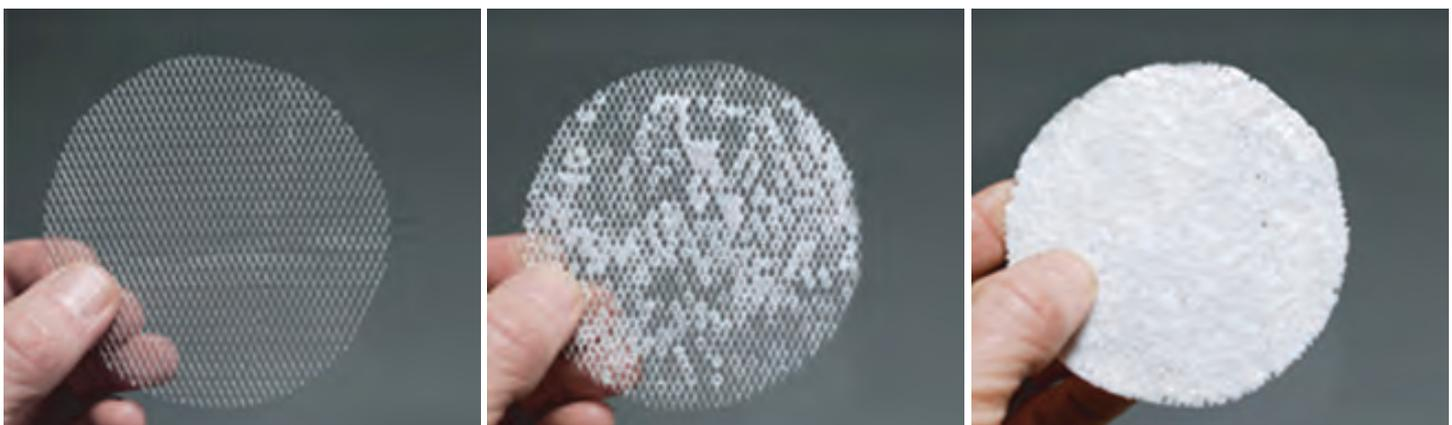
Fig. 7, "GEOtube", vertical salt deposit building skin, crystallisation tests, Faulders Studio
