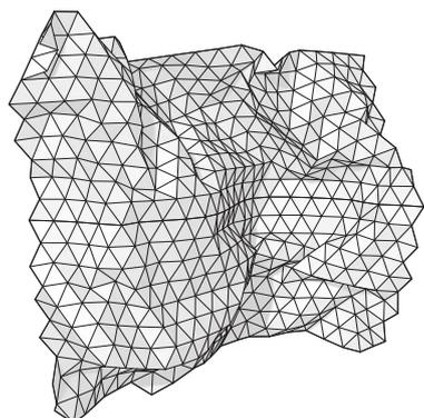
Crumpling of surface based on panel equalateralisation using Kangaroo Physics. Force objects include gravity, springs and hinge angles. Anchor points are based on the meeting between floors
