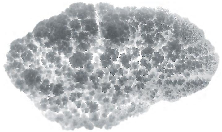
Fig. 43, Salt crystallisation test on felt substrate, growth span: 1 week
