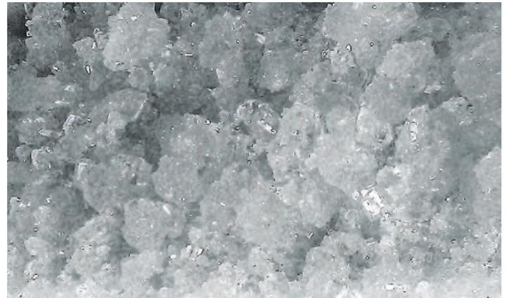
Fig. 44, Salt crystallisation test on felt substrate, growth span: 1 week, close up shot
