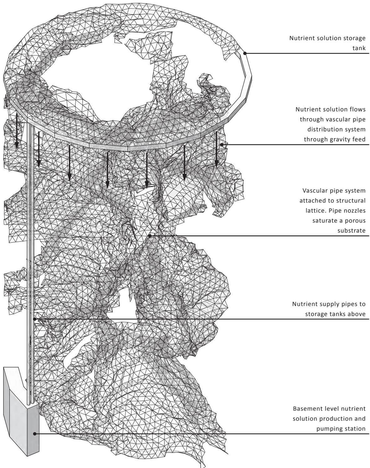
Fig. 128, nutrient distribution system
