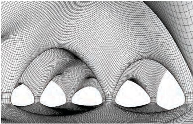
Fig. 46, Kangaroo springs + unary force + anchor points, catenary model generated through Kangaroo (Grasshopper plug-in, Rhino)
