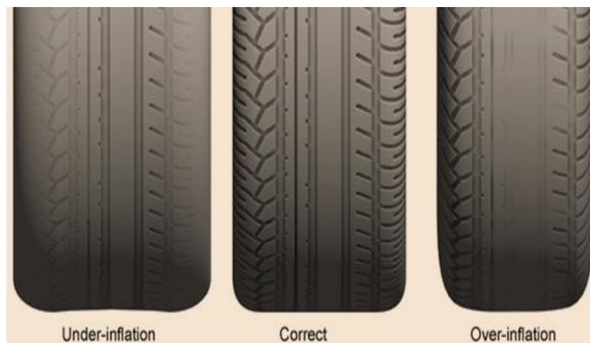
Figure 11: Typical tyre wear patterns observed for different tyre inflation pressures [18].
