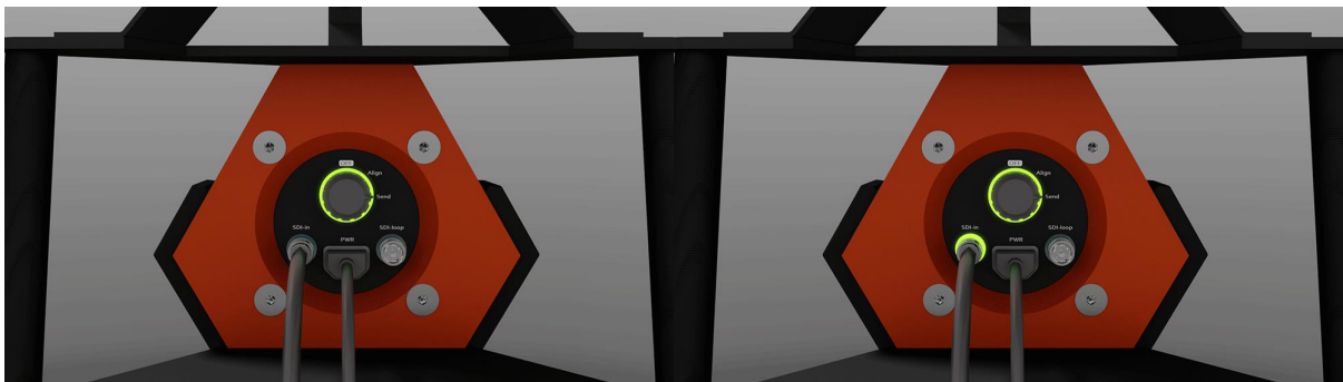
Figure 49 No SDI signal to the left and received SDI signal in to the right
