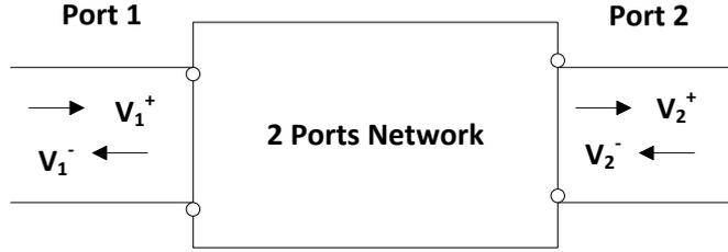
Figure A.1: Incident and scattered voltage waves in a 2-port network
