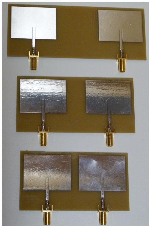
Figure 3.6: Manufactured antenna arrays: 3 different designs for 3 different coupling values
