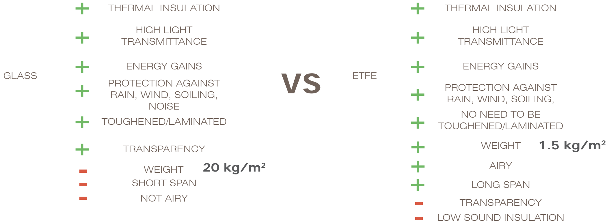
Figure 34 Pros and cons of glass and ETFE membrane
