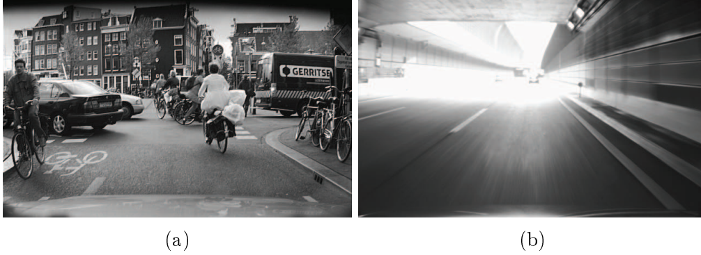
Figure 2.11: Illustration of system verification challenges as seen by a vision sensor. (a) One of the many possible complex traffic situations. (b) The sensor is partially blinded when exiting the tunnel.
