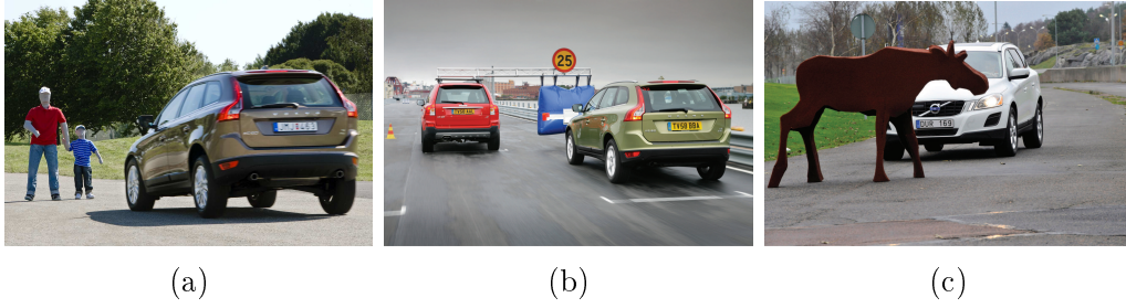
Figure 3.2: Non-destructive tests in collision and near-collision scenarios where (a) shows stationary pedestrian dummies of both adult and child size, (b) shows an inflatable moving object representing a moving vehicle and (c) shows an artificial object representing a moose.
