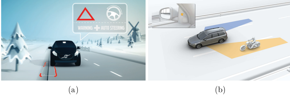
Figure 2.6: (a) A lane guidance system detects the lane markings and warns the driver (LDW), or applies a steering wheel torque (LKA), when crossing the lane boundary. (b) The colored zones visualize the blind spots, i.e. the zones not visible to the driver through the rear view mirrors. LCA indicates that an obstacle is present in the blind spot by lighting a small lamp close to the rear view mirror.
