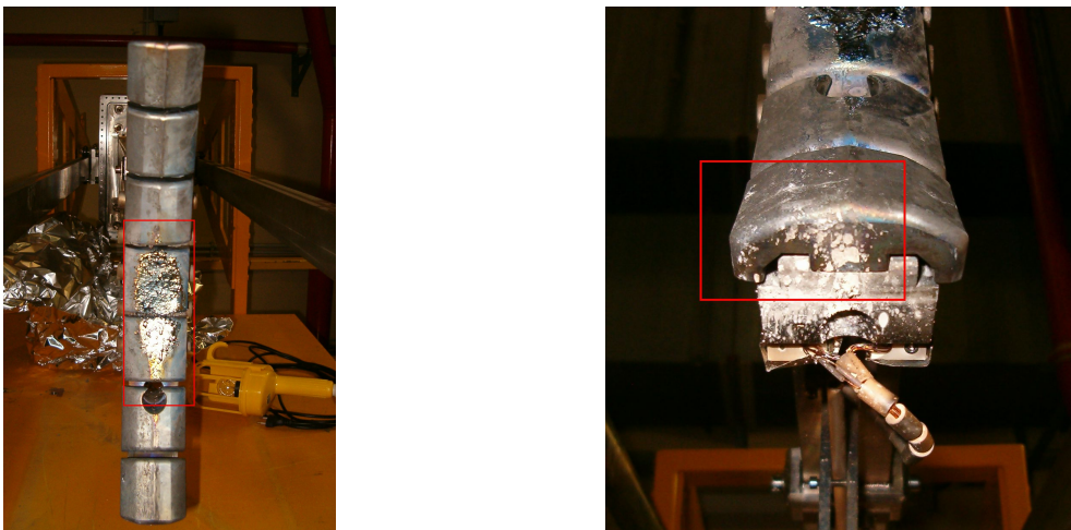
Figure 3.2: Effects of a disruption on Frascati Tokamak Upgrade (FTU) first wall (Photo credits: G.Mazzitelli)
